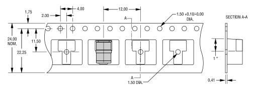
TOLERANCES: ±0.13 UNLESS OTHERWISE SPECIFIED DIMENSIONS: MILLIMETERS
