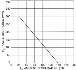
Fig. 6 Max Power Dissipation vs. Ambient Temperature
