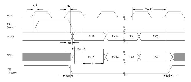
Figure 11: Serial Port Data Timing
