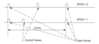
Figure 2: Control Frame Position versus SPOS
