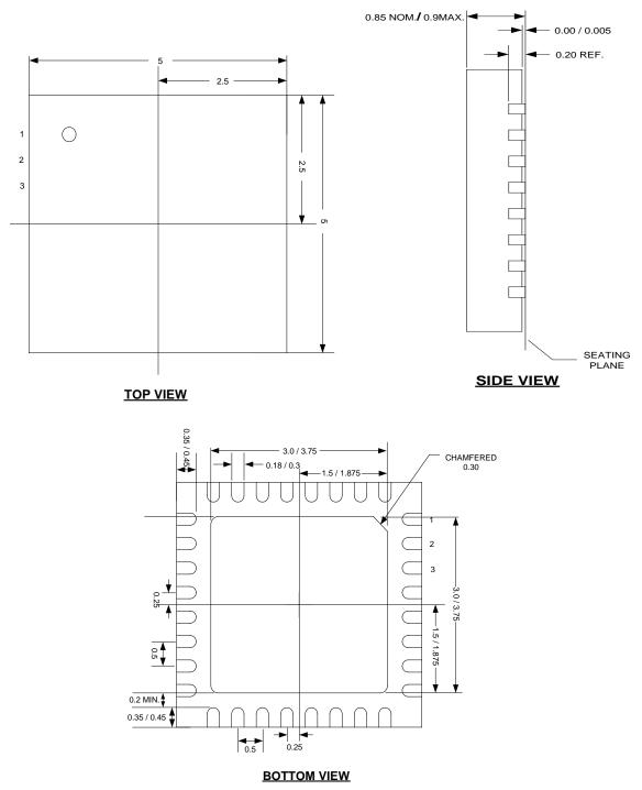
Figure 15: 32-Pin QFN Mechanical Specifications
