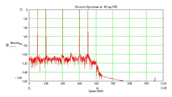
Figure 9: RXD Spectrum of 0.5 kHz, 1 kHz, 2 kHz, 3 kHz and 3.5 kHz Tones of Equal Amplitudes
