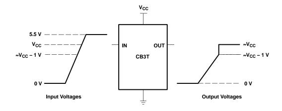
NOTE: If the input high-voltage ( $V_{IH}$ ) level is greater than or equal to  $V_{CC}$  – 1 V and less than or equal to 5.5 V, the output high-voltage ( $V_{OH}$ ) level is equal to approximately the  $V_{CC}$  voltage level.
