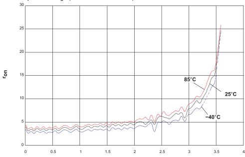
Figure 1.  $r_{ON}$  vs.  $V_{I}$ ,  $V_{CC}$  = 5 V
