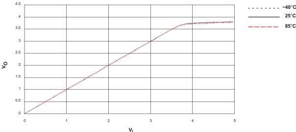
Figure 4.  $V_0$  vs  $V_1$ ,  $V_{CC} = 5$  V
