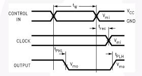
Propagation Delay. Pulse Width and  $t_{rec}$  Waveforms
