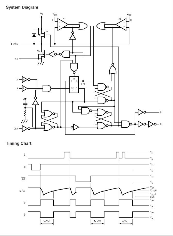
74VHC221A Dual Non-Retriggerable Monostable Multivibrator
