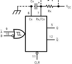
**Note A:** Cx, Rx, Dx are external Capacitor, Resistor, and Diode, respectively.
