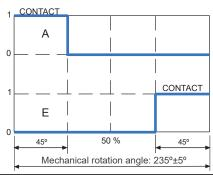
Power rating: 24V / 15mA ON position resistance:  $\leq 5\Omega$  Insulation resistance:  $\geq$  30M $\Omega$
