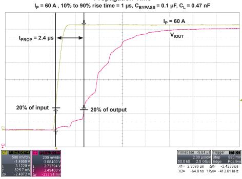
**Propagation Time**  $I_{P} = 60 \text{ A}$  10% to 90% rise time = 1 us Cryston = 0.1 uF Cr = 0.47 nF
