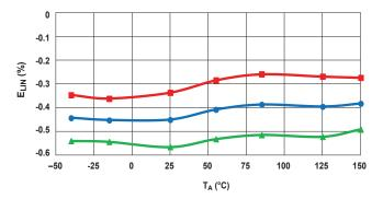
Magnetic Offset Error versus Ambient Temperature
