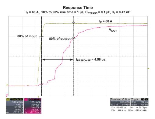
$\label{eq:RiseTime} \begin{array}{l} \textbf{Rise Time} \\ \textbf{I}_{p} = 60 \text{ A} \text{ , } 10\% \text{ to } 90\% \text{ rise time = 1 } \mu\text{s} \text{ , } \textbf{C}_{\text{BYPASS}} = 0.1 \ \mu\text{F} \text{, } \textbf{C}_{\text{L}} = 0.47 \ \text{nF} \end{array}$
