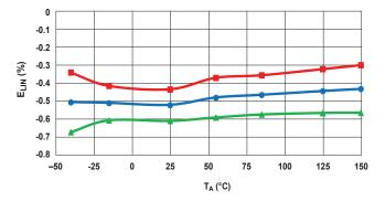
Magnetic Offset Error versus Ambient Temperature
