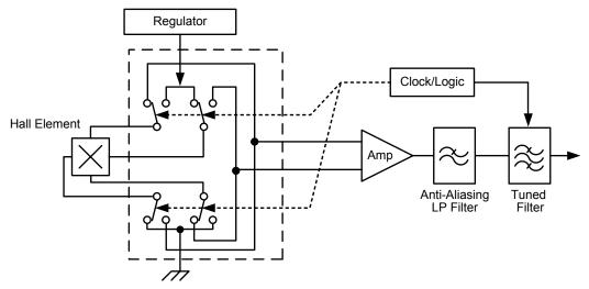
Figure 3: Concept of Chopper Stabilization Technique
