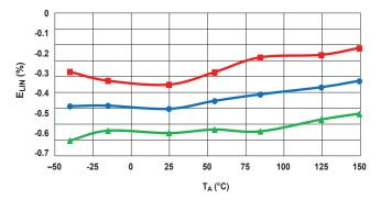
**Total Output Error versus Ambient Temperature**
