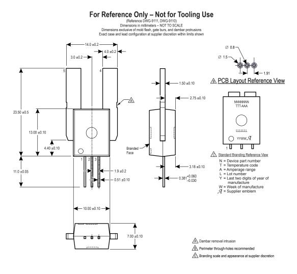
Creepage distance, current terminals to signal pins: 7.25 mm Clearance distance, current terminals to signal pins: 7.25 mm Package mass: 4.63 g typical
