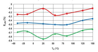
Total Output Error versus Ambient Temperature
