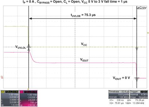
UVLO Enable Time ( $t_{UVLOE}$ ) I<sub>P</sub> = 0 A , C<sub>BYPASS</sub> = Open, C<sub>L</sub> = Open, V<sub>CC</sub> 5 V to 3 V fall time = 1 µs
