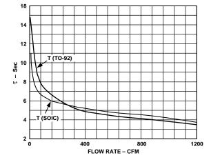
Figure 2. Thermal Response vs. Air Flow Rate
