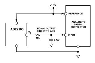
Figure 1. Application Circuit
