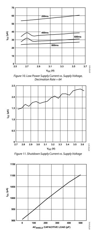
Figure 12. Supply Current vs. Capacitive Load on ACSHIELD
