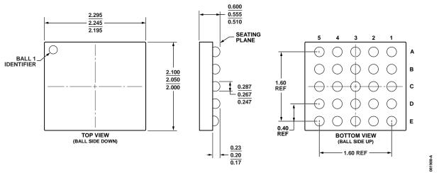
Figure 62. 25-Ball Wafer Level Chip Scale Package [WLCSP] (CB-25-3) Dimensions shown in millimeters
