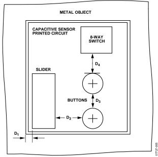
Figure 55. Capacitive Sensor Board, Top View
