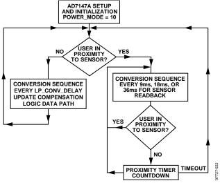
Figure 22. Low Power Mode Operation, AD7147A
