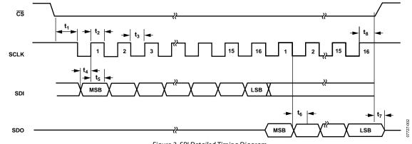
Figure 2. SPI Detailed Timing Diagram
