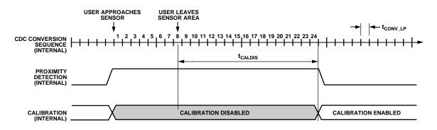
NOTES 1. SEQUENCE CONVERSION TIME t<sub>CONV\_LP</sub> = t<sub>CONV\_FP</sub> + LP\_CONV\_DELAY. 2. PROXIMITY IS SET WHEN THE USER APPROACHES THE SENSOR, AT WHICH TIME THE INTERNAL CALIBRATION IS DISABLED. 3. t<sub>CALDIS</sub> = (t<sub>CONV\_LP</sub> × LP\_PROXIMITY\_CNT × 4).
