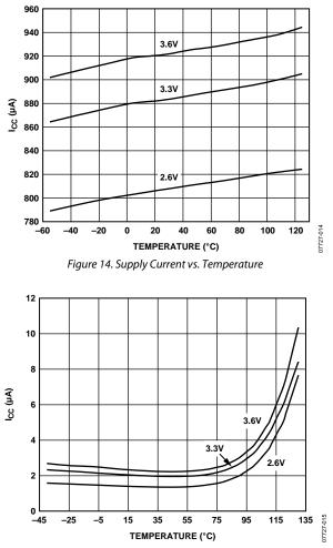
Figure 15. Shutdown Supply Current vs. Temperature
