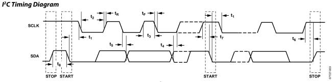
Figure 3. I<sup>2</sup>C Detailed Timing Diagram
