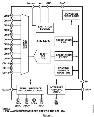
The AD7147A is designed for single electrode capacitance sensors (grounded sensors). There is an active shield output to minimize noise pickup in the sensor.
