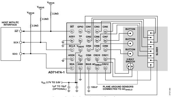
Figure 60. Typical Application Circuit with I<sup>2</sup>C Interface
