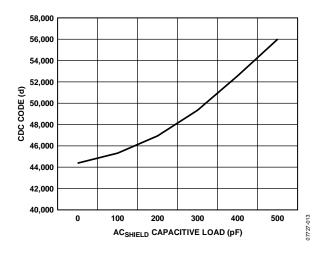
Figure 13. CDC Code vs. Capacitive Load on AC<sub>SHIELD</sub>
