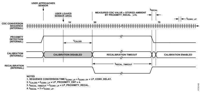
Figure 32. Example of Low Power Mode Proximity Detection with Forced Recalibration  $(LP_PROXIMITY_CNT = 4 \text{ and } LP_PROXIMITY_RECAL = 40)$
