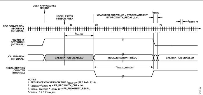
Figure 31. Example of Full Power Mode Proximity Detection with Forced Recalibration (FP\_PROXIMITY\_CNT = 1 and FP\_PROXIMITY\_RECAL = 40)
