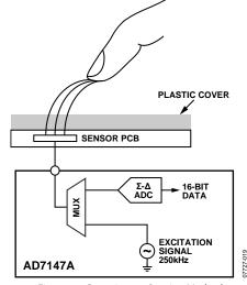
Figure 19. Capacitance-Sensing Method
