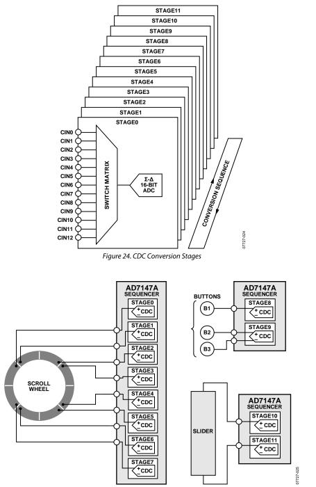
Figure 25. Sequencer Setup for Sensors
