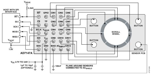
Figure 59. Typical Application Circuit with SPI Interface
