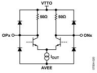
Figure 20. High Speed Output Simplified Schematic
