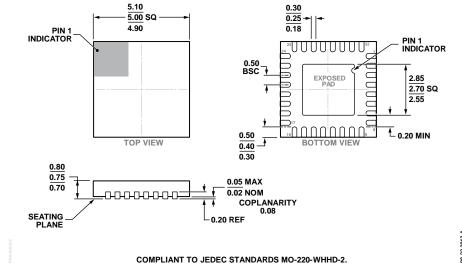
Figure 27. 32-Lead Lead Frame Chip Scale Package [LFCSP] 5 mm × 5 mm Body and 0.75 mm Package Height (CP-32-21) Dimensions shown in millimeters
