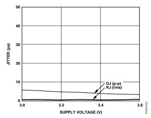
Figure 13. Jitter vs. Supply Voltage
