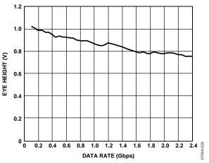
Figure 10. Eye Height vs. Data Rate
