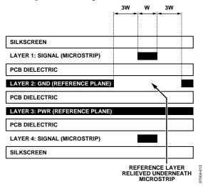
Figure 22. Example Board Stackup
