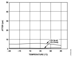
Figure 17. Jitter vs. Temperature
