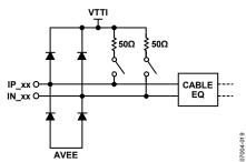
Figure 19. High Speed Input Simplified Schematic
