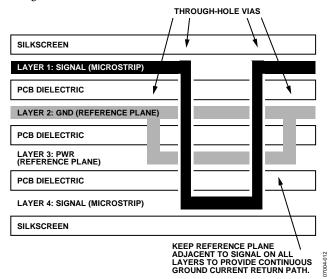
Figure 21. Example Routing of Reference Plane
