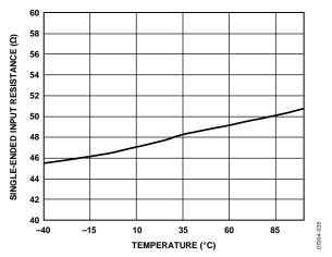
Figure 16. Single-Ended Input Resistance vs. Temperature
