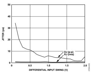
Figure 14. Jitter vs. Differential Input Swing
