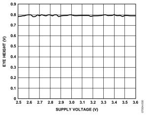
Figure 11. Eye Height vs. Supply Voltage
