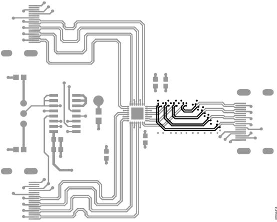
Figure 26. Layout of TMDS Traces
