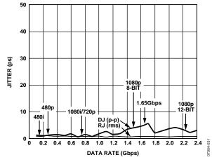
Figure 12. Jitter vs. Data Rate
