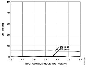
Figure 15. Jitter vs. Input Common-Mode Voltage
