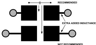
Figure 23. Recommended Pad Outline for Bypass Capacitors
