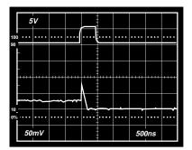
Figure 14. Worst Case 1 LSB Step Change Code  $80_H$  to  $7F_H$ , Upper Trace LD @ 5 V/Div, Lower Trace  $V_{OUT}$  @ 50 mV/Div
