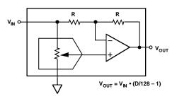
Figure 1. Functional Circuit of One 4-Quadrant Multiplying Channel
