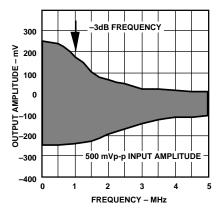
Figure 21. AC Sweep Frequency 500 mV p-p Amplitude Response
