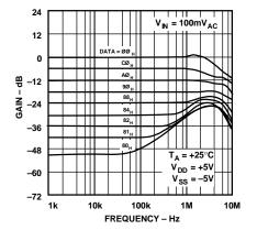
Figure 24. Gain ( $V_{OUT}/V_{IN}$ ) and Feedthrough vs. Frequency
