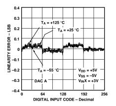
Figure 5. Linearity Error vs. Digital Code vs. Temperature
