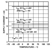
Figure 22. Supply Current vs. Voltage and Temperature
