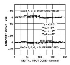
Figure 4. Linearity Error vs. Digital Code
