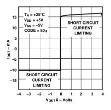
Figure 25. Short Circuit Limit Output Current vs. Voltage
