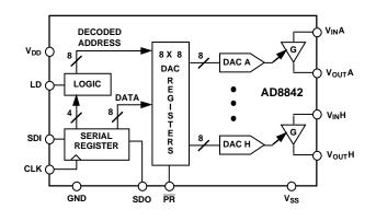
The AD8842 consumes only 95 mW from  $\pm 5$  V power supplies. For single 5 V supply applications consult the DAC-8841. The AD8842 is pin compatible with the 1 MHz multiplying bandwidth DAC8840. The AD8842 is available in 24-pin plastic DIP and surface mount SOL-24 packages.
