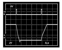
Figure 16. Settling Time—Upper Trace LD @ 5 V/Div, Lower Trace V<sub>OUT</sub> @ 2 V/Div
