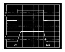
Figure 13. Pulse Response—Upper Trace  $V_{IN}$  @ 2 V/Div Lower Trace  $V_{OUT}$  @2 V/Div
