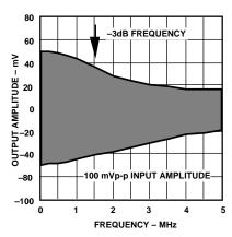
Figure 20. AC Sweep Frequency 100 mV p-p Amplitude Response
