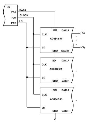
Figure 32. Three-Wire Interface Updates Multiple AD8842s
