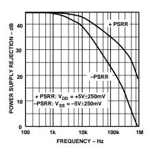
Figure 23. PSRR vs. Frequency
