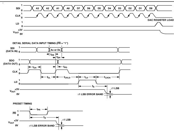
Figure 3. Timing Diagram
