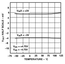
Figure 6. V<sub>OUT</sub> Half Scale (80<sub>H</sub>) vs. Temperature
