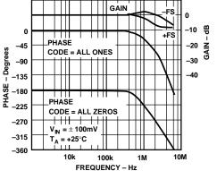
Figure 10. Gain and Phase vs. Frequency (Code =  $00_H$  or FF<sub>H</sub>)
