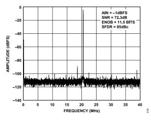
Figure 13. Single-Tone 16k FFT with f<sub>IN</sub> = 140 MHz, f<sub>SAMPLE</sub> = 80 MSPS
