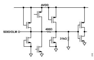
Figure 49. Equivalent SDIO/OLM Input Circuit
