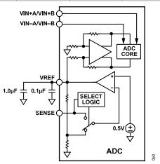
Figure 57. Internal Reference Configuration
