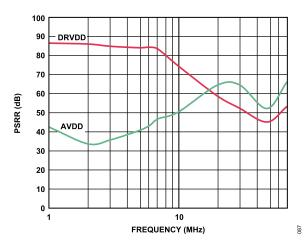
Figure 44. PSRR vs. Frequency,  $f_{CLK}$  = 125 MHz,  $f_{SAMPLE}$  = 125 MSPS
