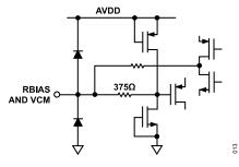
Figure 52. Equivalent RBIAS and VCM Circuit
