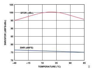
Figure 19. SNR/SFDR vs. Temperature, f<sub>IN</sub> = 10.3 MHz, f<sub>SAMPLE</sub> = 80 MSPS
