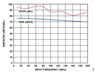
Figure 18. SNR/SFDR vs. f<sub>IN</sub>, f<sub>SAMPLE</sub> = 80 MSPS
