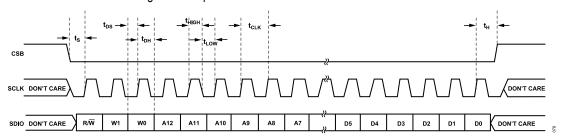
Figure 74. Serial Port Interface Timing Diagram
