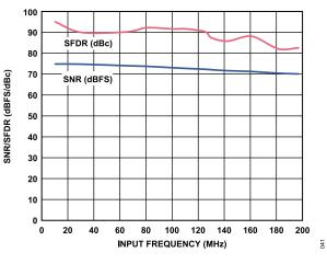
Figure 39. SNR/SFDR vs. f<sub>IN</sub>, f<sub>SAMPLE</sub> = 125 MSPS
