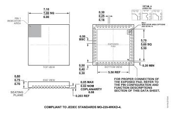
Figure 77. 48-Lead Lead Frame Chip Scale Package [LFCSP] 7 mm × 7 mm Body and 0.75 mm Package Height (CP-48-13) Dimensions shown in millimeters
