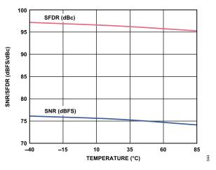
Figure 40. SNR/SFDR vs. Temperature, f<sub>IN</sub> = 10.3 MHz, f<sub>SAMPLE</sub> = 125 MSPS
