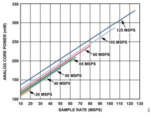
Figure 69. Analog Core Power vs. f<sub>SAMPLE</sub> for f<sub>IN</sub> = 10.3 MHz
