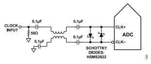
Figure 63. Balun-Coupled Differential Clock (Up to 1 GHz)
