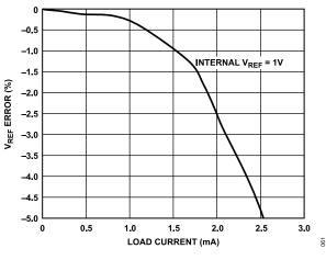
Figure 60. V<sub>REF</sub> Error vs. Load Current
