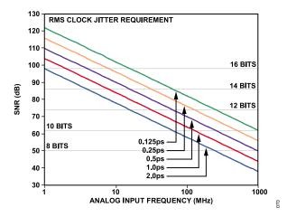
Figure 68. Ideal SNR vs. Input Frequency and Jitter
