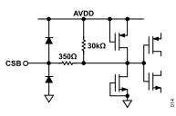
Figure 53. Equivalent CSB Input Circuit
