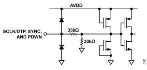
Figure 51. Equivalent SCLK/DTP, SYNC, and PDWN Input Circuit
