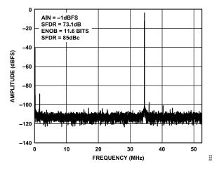
Figure 23. Single-Tone 16k FFT with f<sub>IN</sub> = 140 MHz, f<sub>SAMPLE</sub> = 105 MSPS
