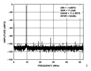
Figure 24. Single-Tone 16k FFT with f<sub>IN</sub> = 200 MHz, f<sub>SAMPLE</sub> = 105 MSPS
