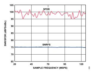
Figure 45. SNR/SFDR vs. Encode, f<sub>IN</sub> = 9.7 MHz, f<sub>SAMPLE</sub> = 125 MSPS
