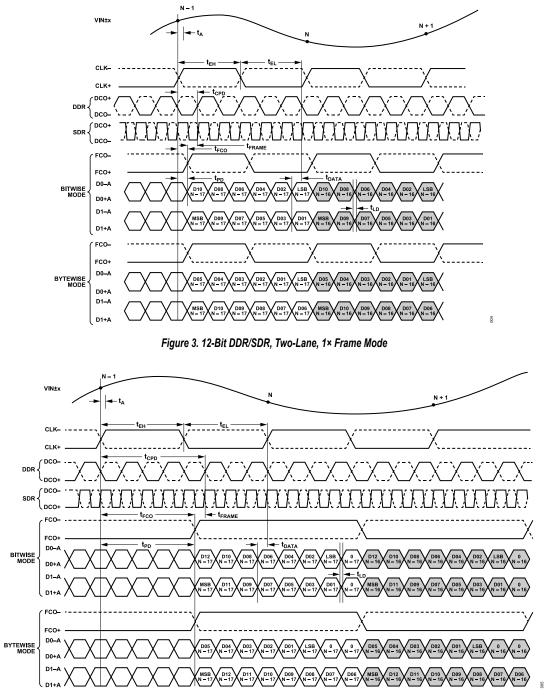
Figure 4. 16-Bit DDR/SDR, Two-Lane, 2× Frame Mode
