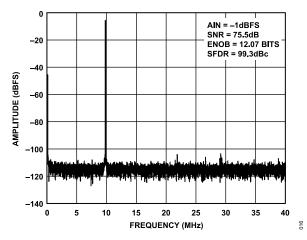
Figure 10. Single-Tone 16k FFT with f<sub>IN</sub> = 9.7 MHz, f<sub>SAMPLE</sub> = 80 MSPS
