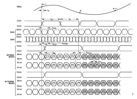
Figure 5. 12-Bit DDR/SDR, Two-Lane, 2× Frame Mode
