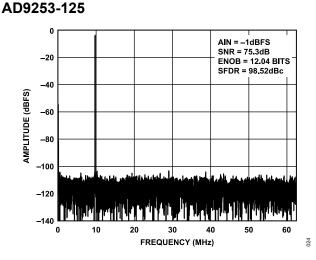
Figure 30. Single-Tone 16k FFT with f<sub>IN</sub> = 9.7 MHz, f<sub>SAMPLE</sub> = 125 MSPS
