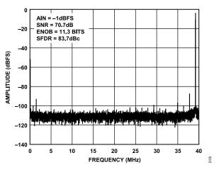
Figure 14. Single-Tone 16k FFT with f<sub>IN</sub> = 200 MHz, f<sub>SAMPLE</sub> = 80 MSPS
