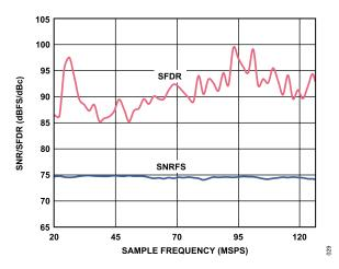
Figure 46. SNR/SFDR vs. Encode,  $f_{IN}$  = 70 MHz,  $f_{SAMPLE}$  = 125 MSPS
