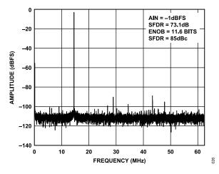
Figure 33. Single-Tone 16k FFT with f<sub>IN</sub> = 140 MHz, f<sub>SAMPLE</sub> = 125 MSPS
