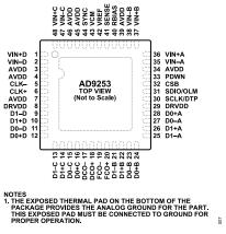
Figure 9. 48-Lead LFCSP Pin Configuration, Top View
