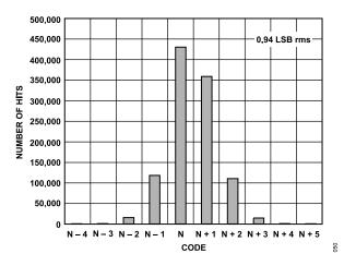
Figure 43. Input-Referred Noise Histogram, f<sub>SAMPLE</sub> = 125 MSPS
