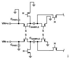
Figure 55. Switched-Capacitor Input Circuit
