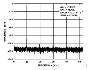
Figure 20. Single-Tone 16k FFT with f<sub>IN</sub> = 9.7 MHz, f<sub>SAMPLE</sub> = 105 MSPS
