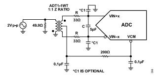
Figure 59. Differential Transformer-Coupled Configuration for Baseband Applications
