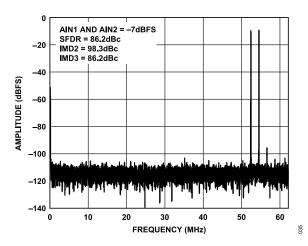
Figure 37. Two-Tone 16k FFT with  $f_{IN1}$  = 70.5 MHz and  $f_{IN2}$  = 72.5 MHz,  $f_{SAMPLE}$ = 125 MSPS
