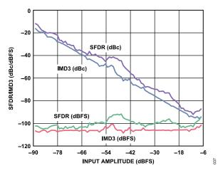
Figure 27. Two-Tone SFDR/IMD3 vs. Input Amplitude (AIN) with  $f_{IN1} = 70.5$  MHz and  $f_{IN2} = 72.5$  MHz,  $f_{SAMPLE} = 105$  MSPS
