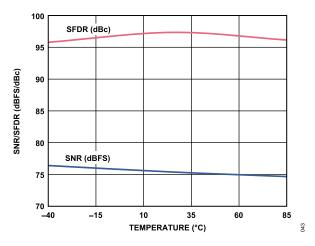
Figure 29. SNR/SFDR vs. Temperature, f<sub>IN</sub> = 10.3 MHz, f<sub>SAMPLE</sub> = 105 MSPS
