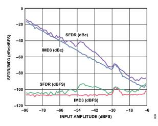
Figure 38. Two-Tone SFDR/IMD3 vs. Input Amplitude (AIN) with  $f_{IN1} = 70.5$  MHz and  $f_{IN2} = 72.5$  MHz,  $f_{SAMPLE} = 125$  MSPS
