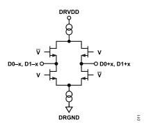
Figure 50. Equivalent Digital Output Circuit
