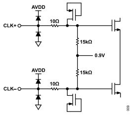
Figure 48. Equivalent Clock Input Circuit
