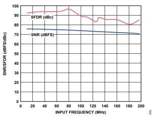
Figure 28. SNR/SFDR vs. f<sub>IN</sub>, f<sub>SAMPLE</sub> = 105 MSPS
