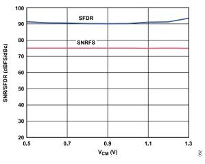
Figure 56. SNR/SFDR vs. Common-Mode Voltage,  $f_{IN}$  = 9.7 MHz,  $f_{SAMPLE}$  = 125 MSPS
