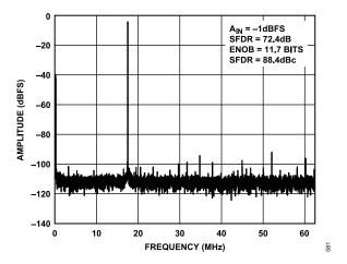
Figure 35. Single-Tone 16k FFT with f<sub>IN</sub> = 140 MHz at f<sub>SAMPLE</sub> = 122.88 MSPS
