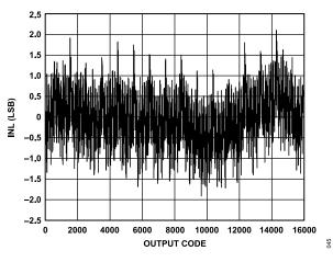
Figure 41. INL, f<sub>IN</sub> = 9.7 MHz, f<sub>SAMPLE</sub> = 125 MSPS
