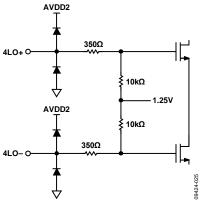
Figure 25. Equivalent 4LO Input Circuit
