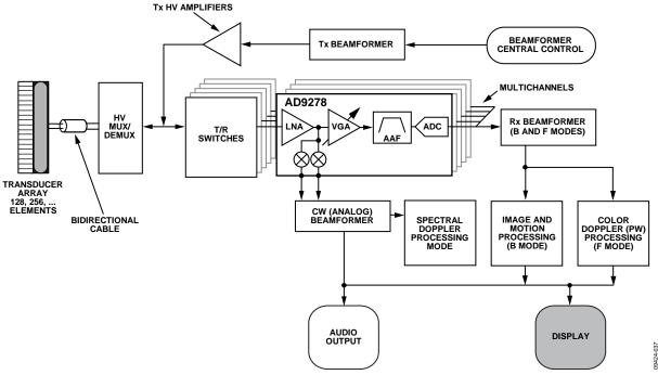
Figure 37. Simplified Ultrasound System Block Diagram
