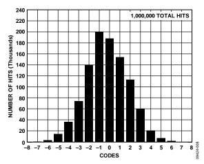
Figure 8. Output-Referred Noise Histogram, GAIN+ = 1.6 V
