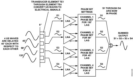
Figure 64. Simplified Example of the AD9278 Phase Shifter
