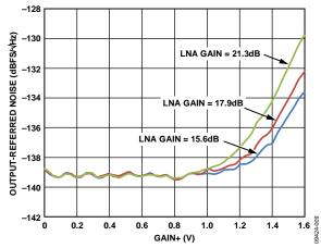
Figure 10. Short-Circuit, Output-Referred Noise vs. GAIN+
