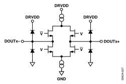
Figure 27. Equivalent Digital Output Circuit
