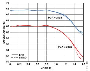
Figure 12. SNR/SINAD vs. GAIN+, AIN = -45 dBm
