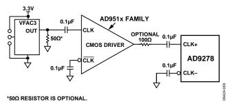
Figure 54. Single-Ended 3.3 V CMOS Sample Clock
