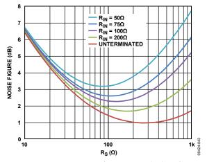
Figure 46. Noise Figure vs.  $R_5$  for Various Fixed Values of  $R_{IN}$ , Active Termination Matched Inputs,  $V_{GAIN} = 1.6 \text{ V}$
