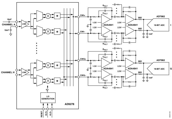
Figure 63. Typical Connection Interface for I/Q Outputs in CW Mode
