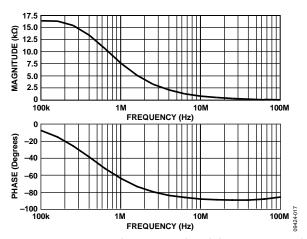
Figure 18. LNA Input Impedance Magnitude and Phase, Unterminated
