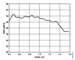
Figure 11. SNR vs. GAIN+, AOUT = -1.0 dBFS
