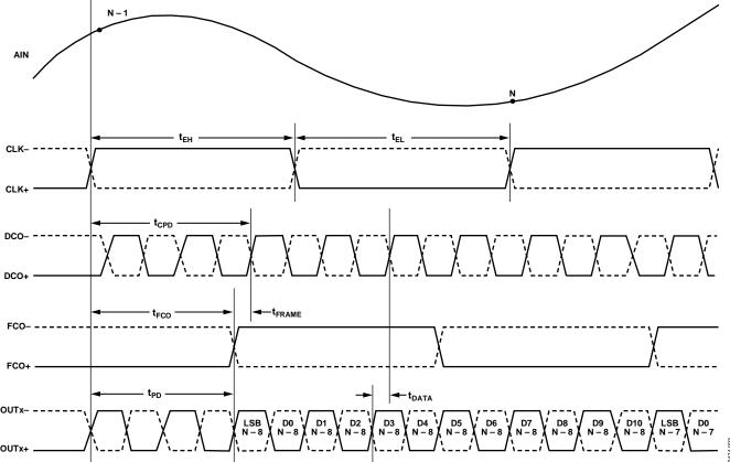
Figure 3. 12-Bit Data Serial Stream, LSB First
