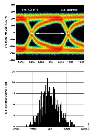
Figure 61. Data Eye for LVDS Outputs in ANSI-644 Mode with Trace Lengths of Greater than 24 Inches on Standard FR-4
