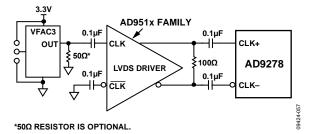
Figure 52. Differential LVDS Sample Clock
