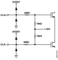
Figure 24. Equivalent Clock Input Circuit
