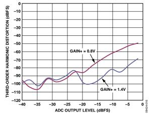
Figure 17. Third-Order Harmonic Distortion vs. ADC Output Level
