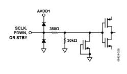
Figure 28. Equivalent SCLK, PDWN, or STBY Input Circuit
