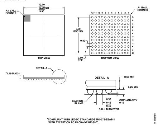
Figure 67. 144-Ball Chip Scale Package, Ball Grid Array [CSP\_BGA] (BC-144-1) Dimensions shown in millimeters
