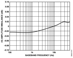
Figure 20. Quadrature (I/Q) Amplitude Error vs. Baseband Frequency
