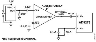
Figure 53. Single-Ended 1.8 V CMOS Sample Clock
