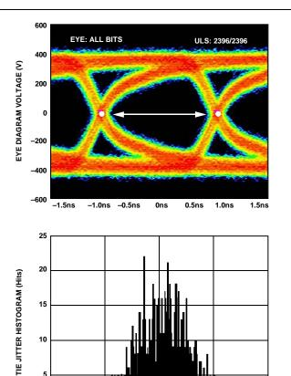
Figure 62. Data Eye for LVDS Outputs in ANSI-644 Mode with 100  $\Omega$  Termination On and Trace Lengths of Greater Than 24 Inches on Standard FR-4
