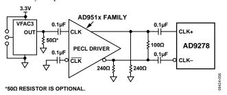
Figure 51. Differential PECL Sample Clock
