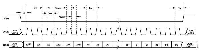
Figure 66. Serial Timing Details
