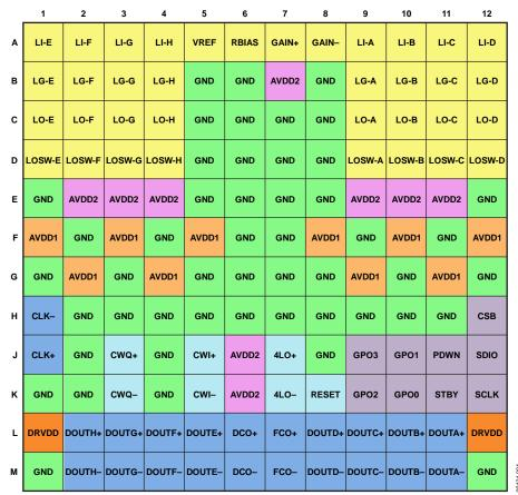
Figure 4. Pin Configuration
