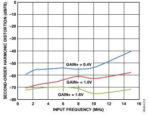
Figure 14. Second-Order Harmonic Distortion vs. Frequency, AOUT = -1.0 dBFS
