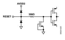
Figure 29. Equivalent RESET Input Circuit
