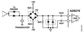
Figure 47. Input Overload Protection
