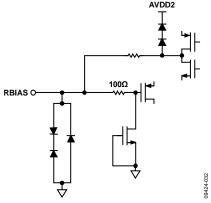
Figure 32. Equivalent RBIAS Circuit
