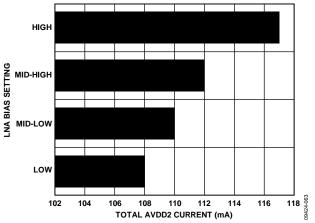
Figure 58. AVDD2 Current at Different LNA Bias Settings,  $f_{SAMPLE} = 40 \text{ MSPS}$
