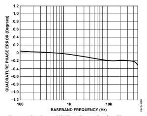
Figure 19. Quadrature (I/Q) Phase Error vs. Baseband Frequency
