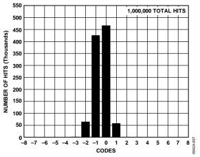
Figure 7. Output-Referred Noise Histogram, GAIN+ = 0.0 V
