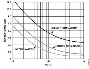
Figure 35. Noise Figure vs.  $R_3$  for Shunt Termination, Active Termination Matched, and Unterminated Inputs,  $V_{GAIN} = 1.6 V$
