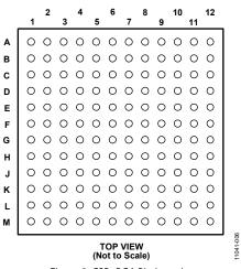
Figure 8. CSP\_BGA Pin Location
