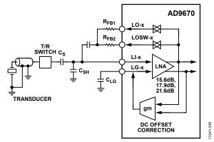
Figure 37. Simplified LNA Input Configuration
