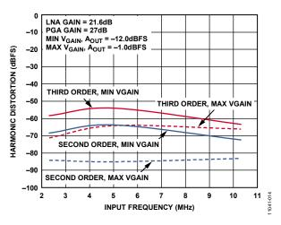
Figure 21. Second-Order and Third-Order Harmonic Distortion vs. Input Frequency,  $A_{OUT} = -1.0 \, dBFS$
