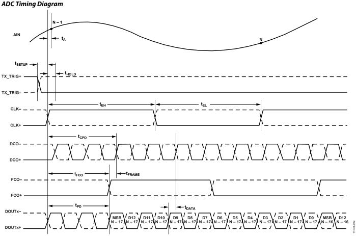
Figure 2. 14-Bit Data Serial Stream (Default, RF Decimator Bypassed, Demodulator Bypassed, Baseband Decimator Bypassed), 1 Channel/Lane Mode, FCO Mode = Word
