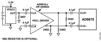
Figure 40. Differential PECL Sample Clock
