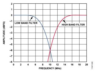
Figure 51. Antialiasing Filter Frequency Response (Frequency Scale Assumes  $f_{ADC} = 2 \times f_{DEC} = 40 \text{ MHz}$ )
