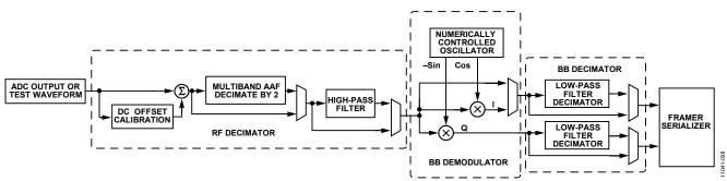
Figure 49. Simplified Block Diagram of a Single Channel of the Demodulator/Decimator
