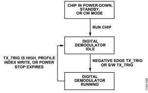
Figure 52. Digital Block Power Saving Scheme
