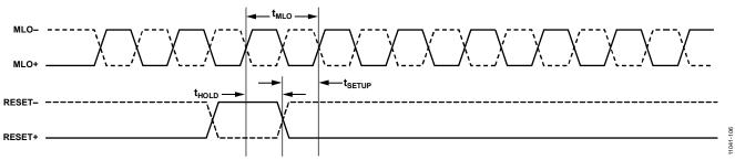
Figure 6. CW Doppler Mode Input MLO $\pm$ , Pulse Asynchronous RESET $\pm$  Timing, 4LO/8LO/16LO Mode
