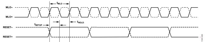
$\textit{Figure 3. CW Doppler Mode Input MLO{\pm}, Continuous Synchronous RESET{\pm} Timing, Sampled on the Falling MLO{\pm} Edge, 4LO Mode Input MLO{\pm}$
