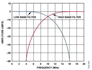
Figure 50. Antialiasing Filter Frequency Response (Frequency Scale Assumes  $f_{ADC} = 2 \times f_{DEC} = 40 \text{ MHz}$ )
