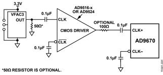
Figure 42. Single-Ended, 1.8 V CMOS Sample Clock
