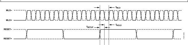
Figure 4. CW Doppler Mode Input MLO±, Continuous Synchronous RESET± Timing, Sampled on the Falling MLO± Edge, 8LO Mode
