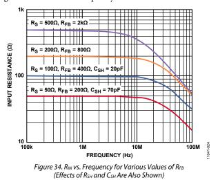
However, as seen for larger  $R_{IN}$  values, parasitic capacitance starts rolling off the signal BW before the LNA produces peaking.  $C_{SH}$  further degrades the match; therefore, do not use  $C_{SH}$  for values of  $R_{IN}$  that are greater than 100  $\Omega$ .
