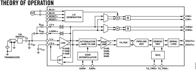
Figure 33. Simplified Block Diagram of a Single Channel
