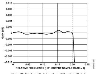
Figure 25. Combined Half-Band 1 and 2 Pass Band Detail; Frequency Relative to HB1 Output Sample Rate
