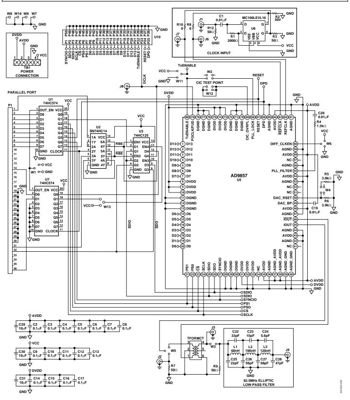
Figure 37. Schematic of AD9857 Evaluation PCB
