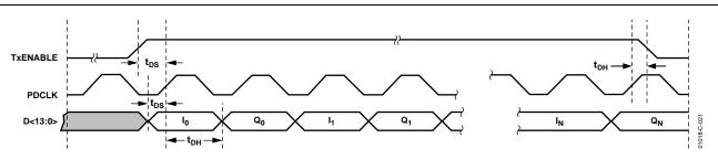
Figure 21. 14-Bit Parallel Port Timing Diagram—Quadrature Modulation Mode
