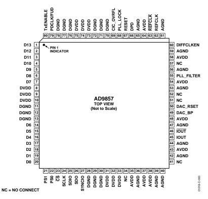
Figure 2. Pin Configuration
