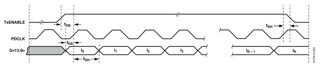
Figure 22. 14-Bit Parallel Port Timing Diagram—Interpolating DAC Mode
