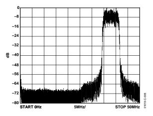
Figure 6. 256-QAM at 38 MHz and 6 MS/s; 48 MHz External Clock with REFCLK Multiplier = 4, CIC Interpolation Rate = 2, 4× Oversampled Data
