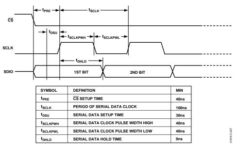
Figure 27. Timing Diagram for Data Write to AD9857
