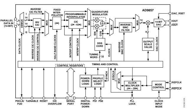
Figure 18. Quadrature Modulation Mode
