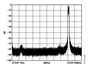
Figure 5. 16-QAM at 65 MHz and 1.28 MS/s; 10.24 MHz External Clock with REFCLK Multiplier = 18, CIC Interpolation Rate = 9, 4× Oversampled Data
