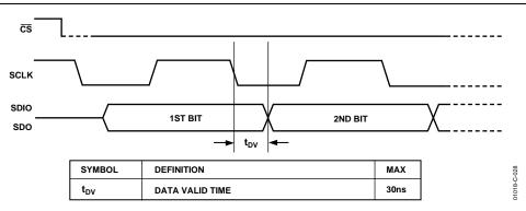
Figure 28. Timing Diagram for Data Read from AD9857
