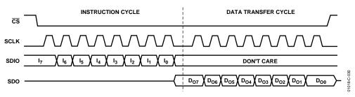
Figure 30. 3-Wire Serial Port Read Timing—Clock Stall Low
