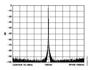
Figure 12. 70.1 MHz Narrow-Band SFDR, 200 MHz External Clock with REFCLK Multiplier Disabled
