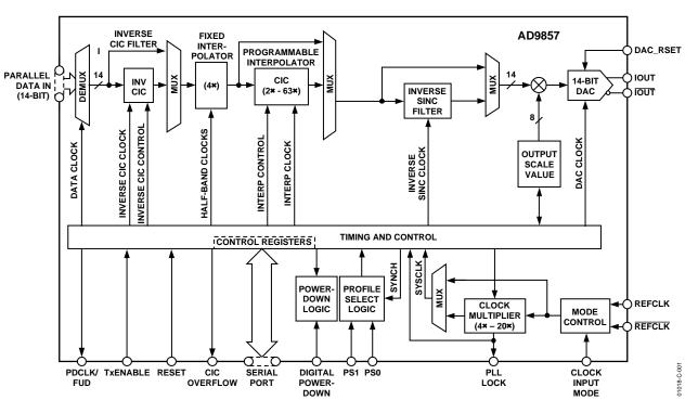
Figure 20. Interpolating DAC Mode
