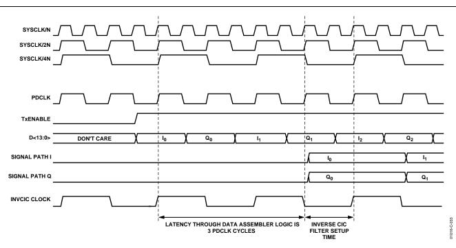
Figure 33. Latency from D<13:0> to Signal Processing Chain, Four PDCLK Cycles
