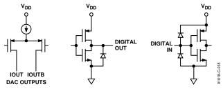
Figure 35. Equivalent I/O Circuits
