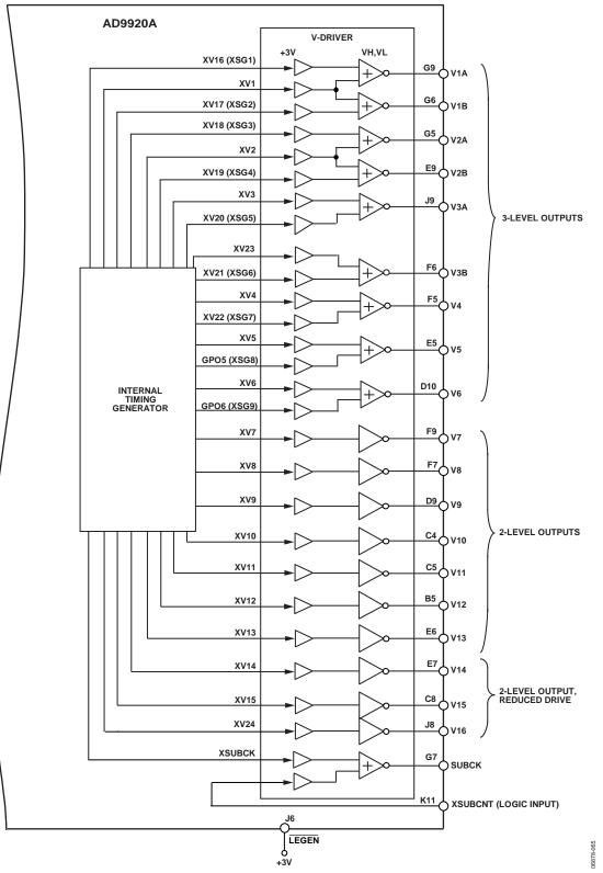
Figure 66. Internal AFETG to V-Driver Connections (19-Channel Mode)
