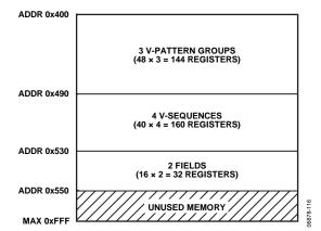
Figure 116. Example Register Configuration
