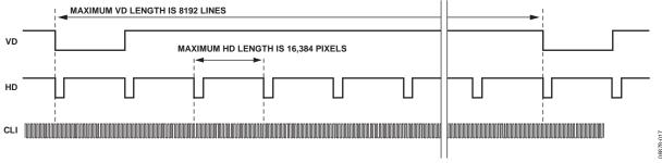
Figure 17. Maximum VD/HD Dimensions
