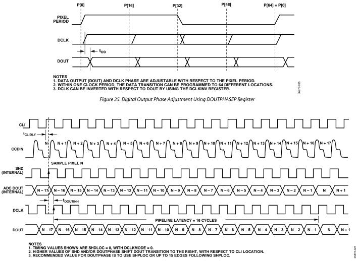
Figure 26. Digital Data Output Pipeline Delay
