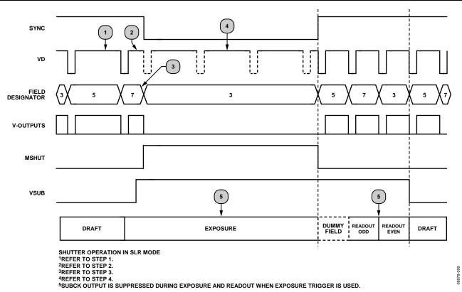
Figure 99. Enhanced SYNC Mode—Manual Shutter Operation, SLR Mode
