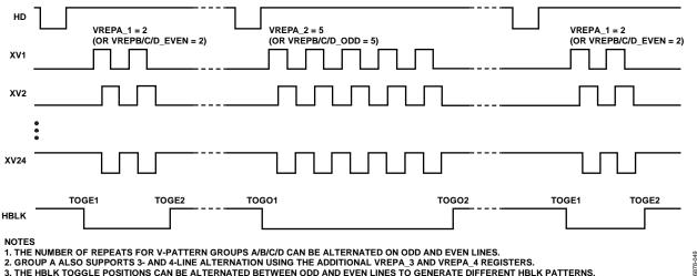
2. GROUP A ALSO SUPPORTS 3- AND 4-LINE ALTERNATION USING THE ADDITIONAL VREPA\_3 AND VREPA\_4 REGISTERS. 3. THE HBLK TOGGLE POSITIONS CAN BE ALTERNATED BETWEEN ODD AND EVEN LINES TO GENERATE DIFFERENT HBLK PATTERNS.
