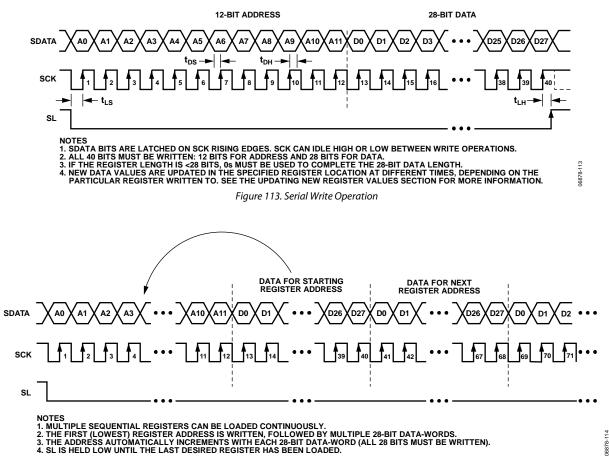
Figure 114. Continuous Serial Write Operation
