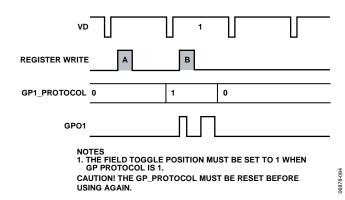
Figure 84. Single-Field Toggles Using GP\_PROTOCOL = 1
