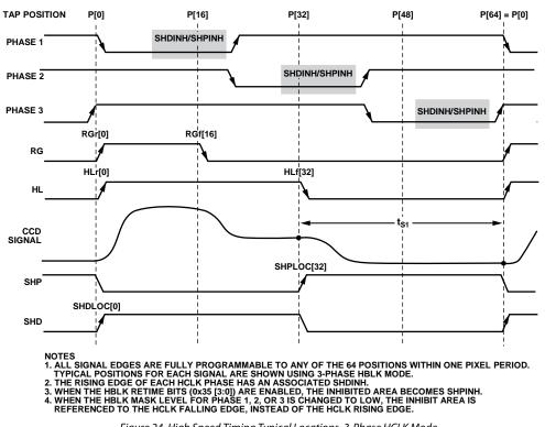
Figure 24. High Speed Timing Typical Locations, 3-Phase HCLK Mode
