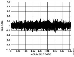
Figure 6. Typical Differential Nonlinearity (DNL) Performance
