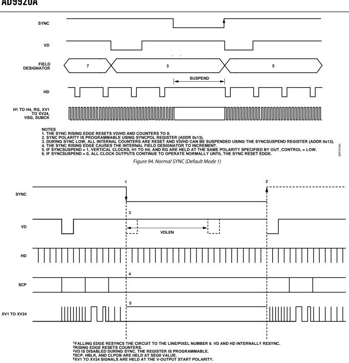
Figure 95. Enhanced SYNC Mode 2 with Vertical Signals Held at VTP Start Value
