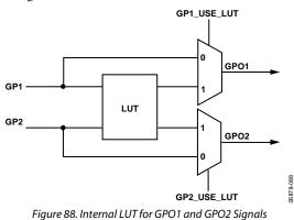
Address 0x7B configures the behavior of the LUT and which signals receive the result. Each 4-bit LUT\_FOR\_GPxy register can realize any logic combination of GPx and GPy. For example, Table 46 shows how the register values of LUT\_FOR\_GP12, Bits[11:8], are determined. XOR, NAND, AND, and OR results are shown, but any 4-bit combination is possible. A simple example of XOR gating is shown in Figure 89.
