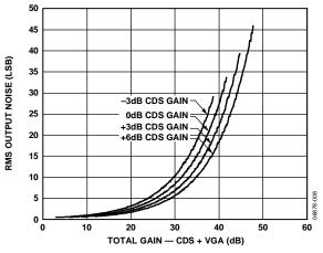
Figure 8. Output Noise vs. Total Gain (CDS + VGA)
