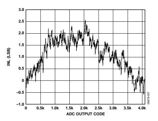
Figure 7. Typical System Integral Nonlinearity (INL) Performance
