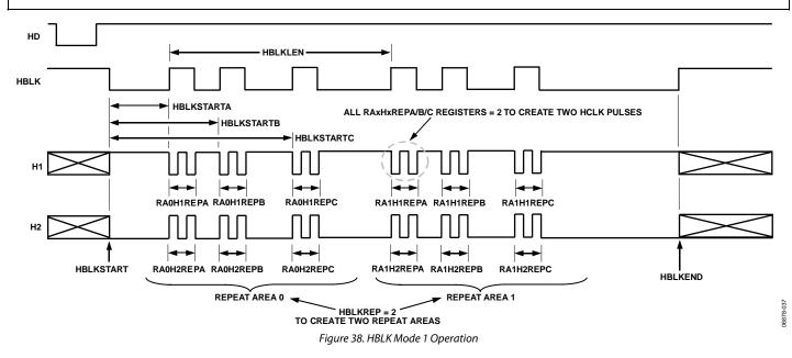
As shown in Figure 38, setting the RAxH1REPA/B/C or RAxH2REPA/B/C register to 0 masks HCLK groups from appearing in a particular repeat area. Figure 37 shows only two repeat areas being used, although six are available. It is possible to program a separate number of repeat area repetitions for H1 and H2, but generally the same value is used for both H1 and H2. Figure 37 shows an example of RA0H1REPA/B/C = RA0H2REPA/B/C = RA1H1REPA/B/C = RA1H2REPA/B/C = 2.
