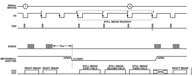
Figure 91. Exposure/Readout Operation Without Using GPO for SG Signal
