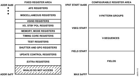
Figure 115. Layout of AD9920A Registers
