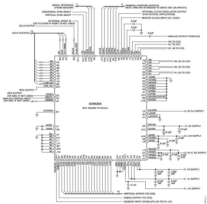
Figure 111. Typical 1.8 V Circuit Configuration in 19-Channel Mode
