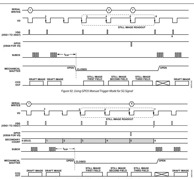
Figure 93. Using GPO5 with Secondary Counter to Control SG Signal
