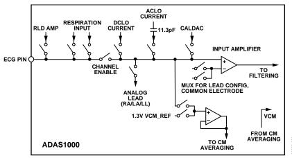
Figure 65. Typical ECG Channel Input Multiplexing
