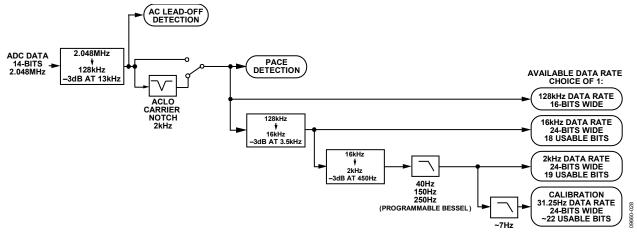
Figure 75. ECG Channel Filter Signal Flow
