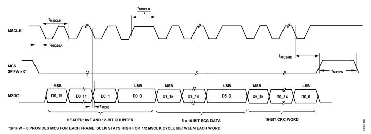
Figure 5. Data Read and Write Timing Diagram for SPIFW = 0, Showing Entire Packet of Data (Header, 5 ECG Words, and CRC Word)
