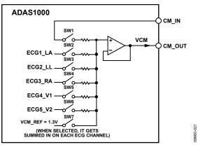
Figure 66. Common-Mode Generation Block
