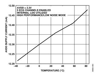
Figure 31. Typical AVDD Supply Current vs. Temperature, Using Internal ADVCDD/DVDD Supplies
