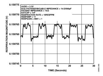
Figure 40. Respiration with 200 m $\Omega$  Impedance Variation, Using External Respiration DAC Driving 1 nF External Capacitor and Measured with a 1 k $\Omega$  Patient Cable
