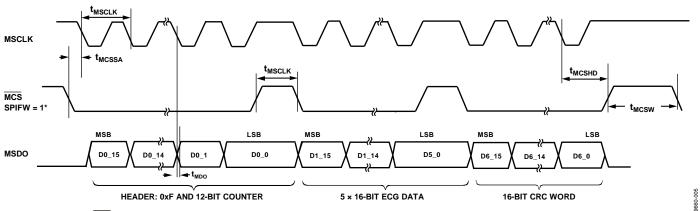
\*SPIFW = 1 PROVIDES  $\overline{MCS}$  FOR EACH FRAME, SCLK STAYS HIGH FOR 1 MSCLK CYCLE BETWEEN EACH WORD.
