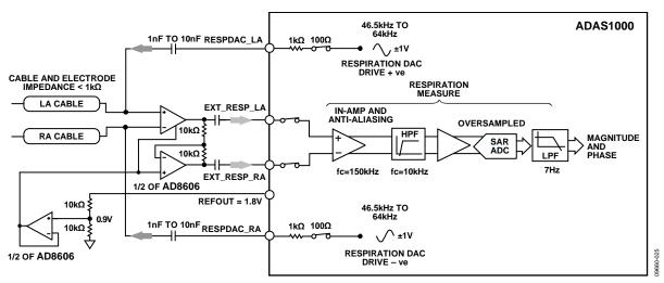
Figure 71. Respiration Using External Capacitor and External Amplifiers
