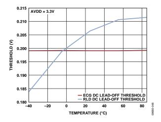
Figure 21. DC Lead-Off Comparator Low Threshold vs. Temperature
