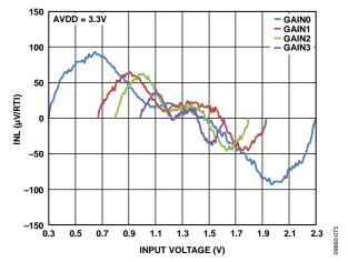
Figure 44. INL vs. Input Voltage Across Gain Setting for 2 kHz Data Rate
