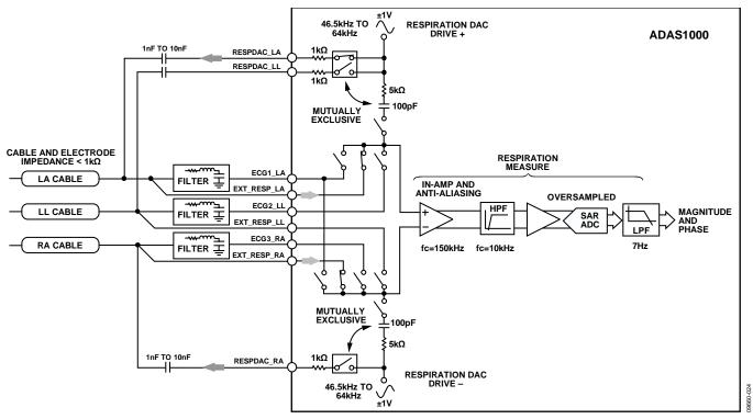
Figure 70. Respiration Measurement Using External Capacitor
