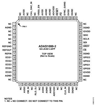
Figure 10. ADAS 1000-2 Companion 64-Lead LQFP Pin Configuration
