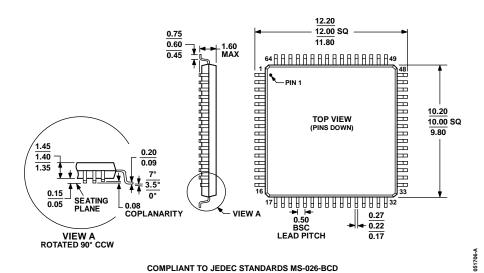
Figure 86. 64-Lead Low Profile Quad Flat Package [LQFP] (ST-64-2) Dimensions shown in millimeters
