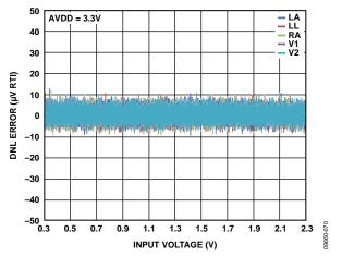
Figure 42. DNL vs. Input Voltage Range Across Electrodes at 25°C
