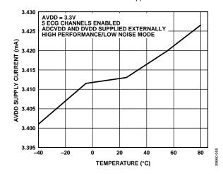
Figure 32. Typical AVDD Supply Current vs. Temperature, Using Externally Supplied ADVCDD/DVDD
