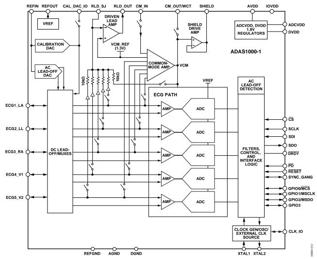
Figure 54. ADAS1000-1 Simplified Block Diagram
