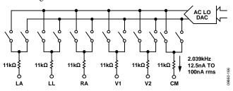
Figure 68. Simplified AC Lead-Off Configuration
