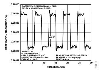
Figure 38. Respiration with 200 m $\Omega$  Impedance Variation, Using External Respiration DAC Driving 100 pF External Capacitor and Measured with a 0  $\Omega$  Patient Cable
