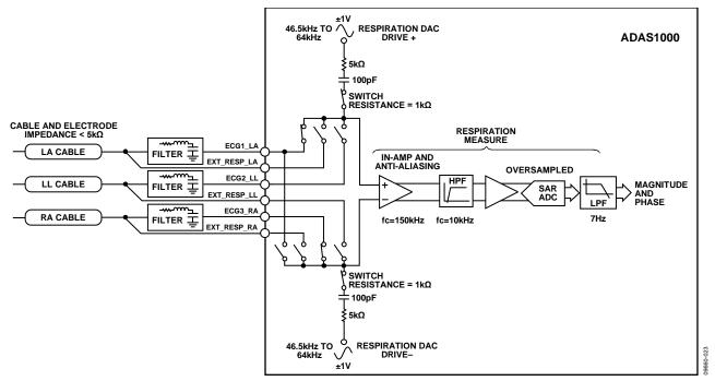
Figure 69. Simplified Respiration Block Diagram
