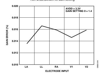
Figure 17. Typical Gain Error Across Channels
