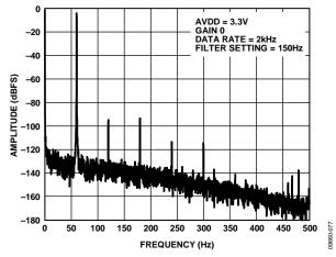
Figure 48. FFT with 60 Hz Input Signal
