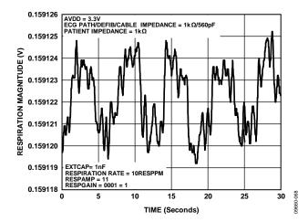
Figure 41. Respiration with 100 m $\Omega$  Impedance Variation, Using External Respiration DAC Driving 1 nF External Capacitor and Measured with a 1 k $\Omega$  Patient Cable
