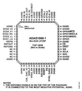
Figure 9. ADAS1000-1 56-Lead LFCSP Pin Configuration
