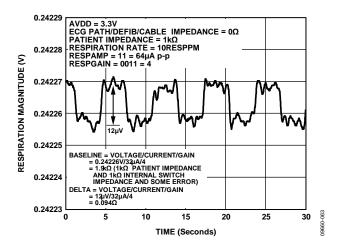
Figure 36. Respiration with 100 m $\Omega$  Impedance Variation, Using Internal Respiration Paths and Measured with a 0  $\Omega$  Patient Cable
