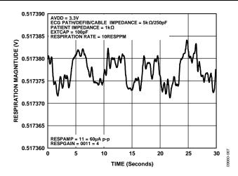
Figure 39. Respiration with 200 m $\Omega$  Impedance Variation, Using External Respiration DAC Driving 100 pF External Capacitor and Measured with a 5 k $\Omega$  Patient Cable
