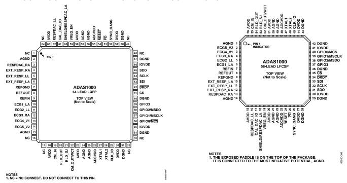
Figure 7. ADAS 1000 64-Lead LQFP Pin Configuration
