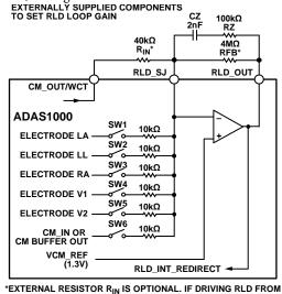
Figure 67. Right Leg Drive—Possible External Component Configuration
