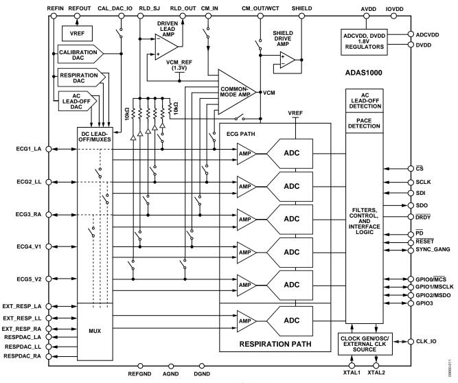
Figure 53. ADAS 1000 Simplified Block Diagram
