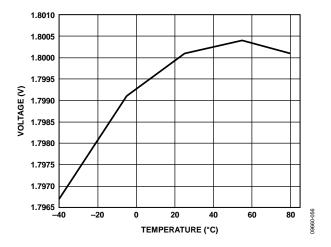
Figure 29. Typical Internal VREF vs. Temperature
