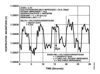
Figure 37. Respiration with 200 m $\Omega$  Impedance Variation, Using Internal Respiration Paths and Measured with a 5 k $\Omega$  Patient Cable
