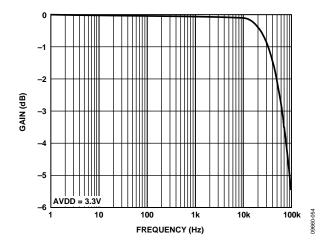
Figure 27. Analog Channel Bandwidth
