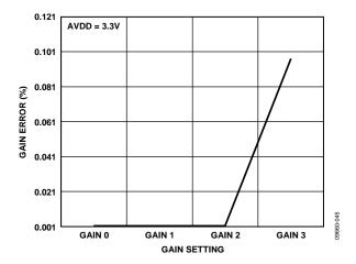
Figure 18. Typical Gain Error vs. Gain
