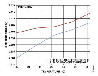
Figure 22. DC Lead-Off Comparator High Threshold vs. Temperature
