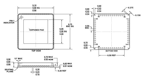
\*FOR PROPER CONNECTION OF THE EXPOSED PAD, REFER TO THE PIN CONFIGURATION AND FUNCTION DESCRIPTIONS SECTION OF THIS DATA SHEET.
