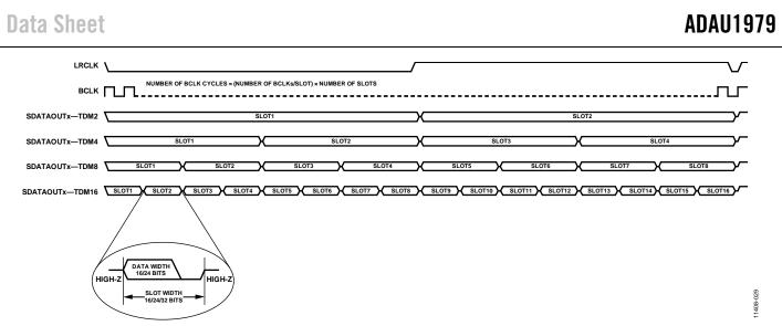
Figure 27. TDM Mode Slot Assignment
