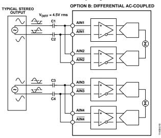
Figure 20. 2-Channel Summing Mode Connection Diagram
