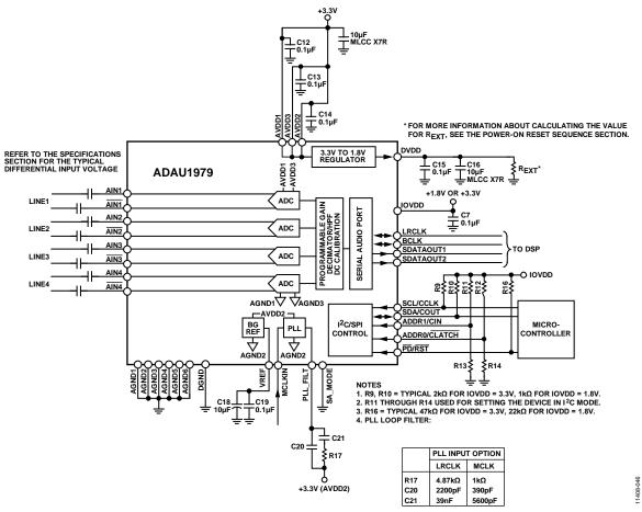
Figure 44. Typical Application Circuit, Four Inputs, I<sup>2</sup>C and I<sup>2</sup>S Mode
