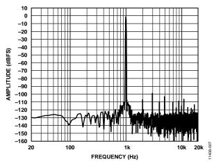
Figure 7. Fast Fourier Transform, –1 dBFS Differential Input
