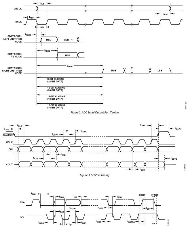
Figure 4. I<sup>2</sup>C Port Timing
