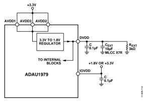
Figure 14. DVDD Regulator Output Connections
