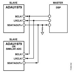
Figure 32. Serial Port Connection Option 5—TDM Mode, DSP Master
