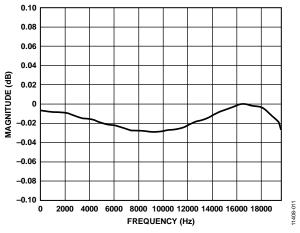
Figure 11. ADC Pass-Band Ripple at  $f_s = 48 \text{ kHz}$
