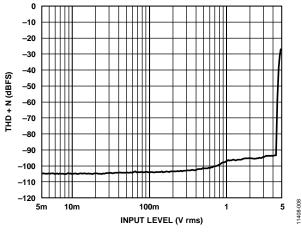
Figure 8. THD + N vs. Input Amplitude
