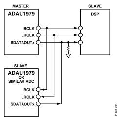
Figure 30. Serial Port Connection Option 3—TDM Mode, ADAU1979 Master
