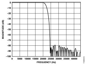
Figure 12. ADC Filter Stop-Band Response at  $f_s = 48 \text{ kHz}$
