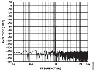
Figure 6. Fast Fourier Transform, 4.5 mV Differential Input at  $f_5 = 48$  kHz
