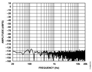
Figure 10. Fast Fourier Transform, No Input
