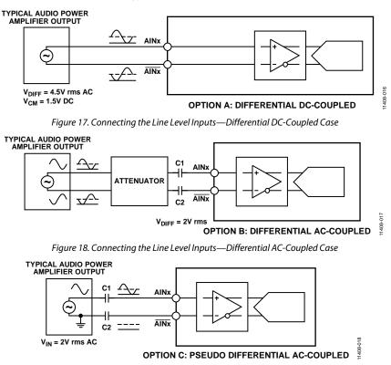
Figure 19. Connecting the Line Level Inputs—Pseudo Differential AC-Coupled Case
