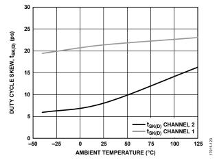
Figure 28. Duty Cycle Skew, t<sub>SK(D)</sub> vs. Ambient Temperature
