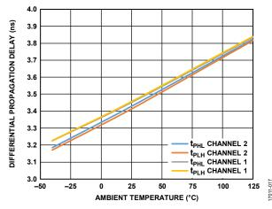
Figure 22. Differential Propagation Delay vs. Ambient Temperature
