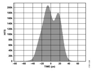
Figure 32. Time Interval Error (TIE) Histogram for  $D_{OUT1\pm}$  at 550 MHz
