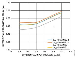
Figure 23. Differential Propagation Delay vs. Differential Input Voltage, VID
