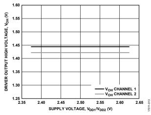
Figure 18. Driver Output High Voltage, VOH vs. Supply Voltage, VDD1/VDD2
