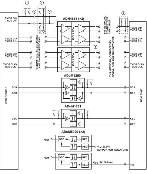
NOTES 1. SUPPLY BIASED TERMINATION 2. AC COUPLING 3. COMMON-MODE BIASING 4. DIFFERENTIAL TERMINATION
