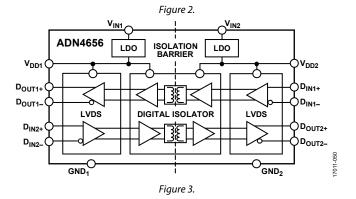
1 on the corresponding LVDS driver output when the inputs are floating, shorted, or terminated but not driven.
