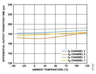
Figure 26. Differential Output Transition Time vs. Ambient Temperature
