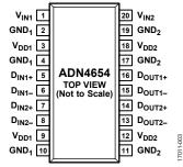
Figure 6. ADN4654 Pin Configuration
