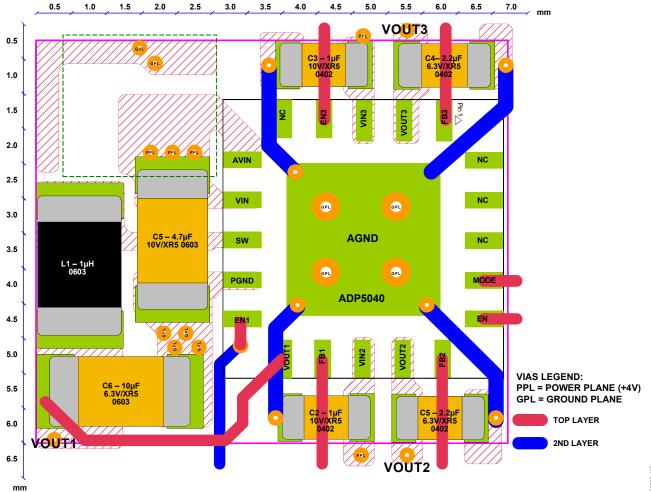
Figure 109. Evaluation Board Layout
