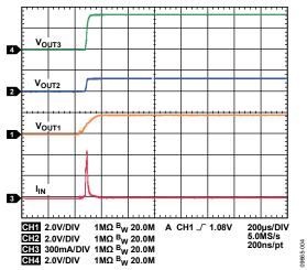
Figure 4. Total Inrush Current, All Channels Started Simultaneously
