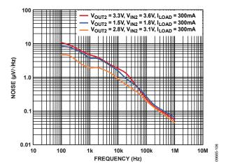
Figure 92. LDO1 Noise Spectrum Across Output Voltage,  $V_{IN} = V_{OUT} + 0.3 V$
