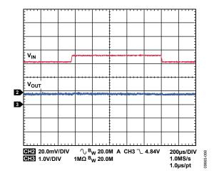
Figure 88. LDO1, LDO2 Response to Line Transient, Input Voltage from 3.3 V to 3.8 V,  $V_{OUT}$  = 1.2 V
