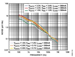
Figure 94. LDO1 vs. LDO2 Noise Spectrum
