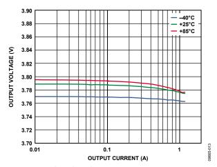
Figure 13. Buck Load Regulation Across Temperature,  $V_{\text{OUTI}} = 3.8 \text{ V}$ , PWM Mode
