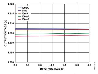
Figure 72. LDO1, LDO2 Line Regulation Across Input Voltage,  $V_{\text{OUT}} = 1.8 \text{ V}$
