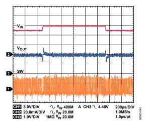
Figure 45. Buck Response to Line Transient, Input Voltage from 4.5 V to 5.0 V,  $V_{\text{OUTI}} = 1.8 \text{ V}$ , PWM Mode
