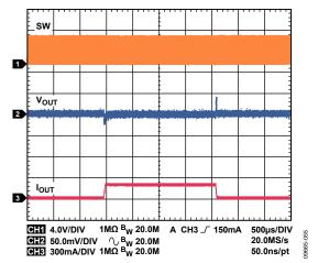
Figure 55. Buck Response to Load Transient,  $I_{OUT1} = 20$  mA to 200 mA,  $V_{OUT1} = 1.8 \text{ V}$ , PWM Mode
