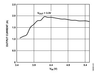
Figure 31. Buck DC Current Capability vs. Input Voltage
