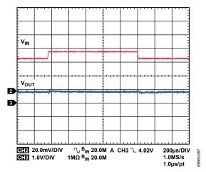
Figure 87. LDO1, LDO2 Response to Line Transient, Input Voltage from 3.3 V to 3.8 V,  $V_{\text{OUT}} = 1.8 \text{ V}$
