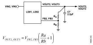
Figure 103. LDOs External Output Voltage Setting
