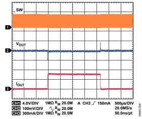
Figure 56. Buck Response to Load Transient,  $I_{OUT1} = 50$  mA to 500 mA,  $V_{OUT1} = 1.8$  V, PWM Mode
