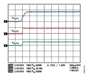
Figure 3. 3-Channel Start-Up Waveforms
