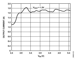
Figure 33. Buck DC Current Capability vs. Input Voltage
