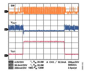
Figure 52. Buck Response to Load Transient,  $I_{OUT1} = 50$  mA to 500 mA,  $V_{OUT1} = 1.2$  V, Auto Mode
