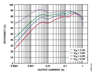
Figure 23. Buck Efficiency vs. Load Current, Across Input Voltage,  $V_{OUT1} = 1.2 V$ , Auto Mode
