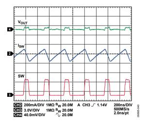
Figure 40. Typical Waveforms, V<sub>OUT1</sub> = 1.2 V, I<sub>OUT1</sub> = 30 mA, PWM Mode
