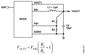
Figure 102. Buck External Output Voltage Setting
