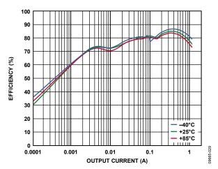
Figure 29. Buck Efficiency vs. Load Current, Across Temperature,  $V_{IN} = 5.0 \text{ V}$ ,  $V_{OUTI} = 1.2 \text{ V}$ , Auto Mode
