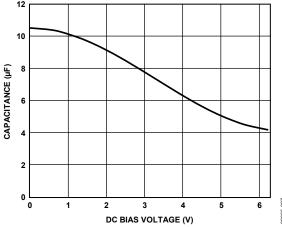
Figure 105. Typical Capacitor Performance
