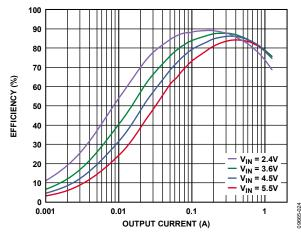
Figure 24. Buck Efficiency vs. Load Current, Across Input Voltage,  $V_{OUTI} = 1.2 \text{ V}$ , PWM Mode
