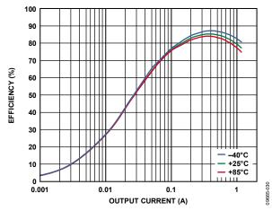
Figure 30. Buck Efficiency vs. Load Current, Across Temperature,  $V_{\text{IN}} = 5.0 \text{ V}, V_{\text{OUTI}} = 1.2 \text{ V}, PWM \text{ Mode}$
