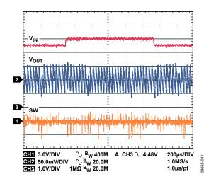
Figure 41. Buck Response to Line Transient, Input Voltage from 4.5 V to 5.0 V,  $V_{OUT1} = 3.3$  V,  $I_{OUT1} = 5$  mA, Auto Mode
