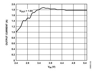
Figure 32. Buck DC Current Capability vs. Input Voltage
