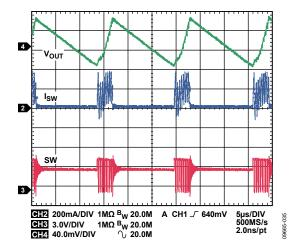
Figure 35. Typical Waveforms,  $V_{OUT1} = 3.3 \text{ V}$ ,  $I_{OUT1} = 30 \text{ mA}$ , Auto Mode
