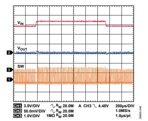
Figure 46. Buck Response to Line Transient, Input Voltage from 4.5 V to 5.0 V,  $V_{\text{OUTI}} = 1.2 \text{ V}$ , PWM Mode
