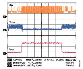
Figure 51. Buck Response to Load Transient,  $I_{OUT1}$  = 20 mA to 200 mA,  $V_{OUT1}$  = 1.2 V, Auto Mode
