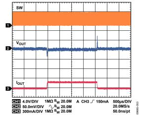
Figure 53. Buck Response to Load Transient,  $I_{OUT1} = 20$  mA to 200 mA,  $V_{OUT1} = 3.3$  V, PWM Mode
