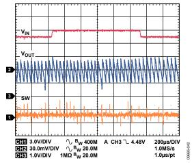
Figure 42. Buck Response to Line Transient, Input Voltage from 4.5 V to 5.0 V,  $V_{OUT1} = 1.8$  V,  $I_{OUT1} = 5$  mA, Auto Mode
