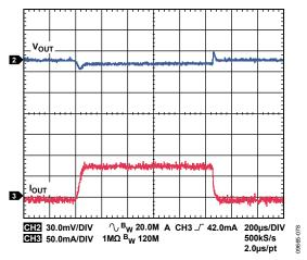
Figure 78. LDO1, LDO2 Response to Load Transient,  $I_{OUT}$  from 1 mA to 80 mA,  $V_{OUT}$  = 3.3 V
