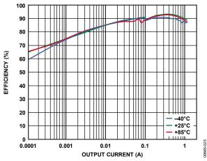
Figure 25. Buck Efficiency vs. Load Current, Across Temperature,  $V_{IN} = 5.0 \text{ V}$ ,  $V_{OUTI} = 3.3 \text{ V}$ , Auto Mode
