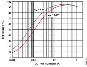
Figure 18. Buck Efficiency vs. Load Current, Across Input Voltage,  $V_{OUTI} = 3.8 \text{ V}$ , PWM Mode
