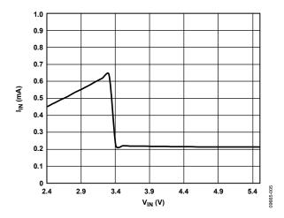
Figure 5. System Quiescent Current (Sum of All the Input Currents) vs. Input Voltage,  $V_{OUT1} = 1.8 \text{ V}$ ,  $V_{OUT2} = V_{OUT3} = 3.3 \text{ V}$  (UVLO = 3.3 V)
