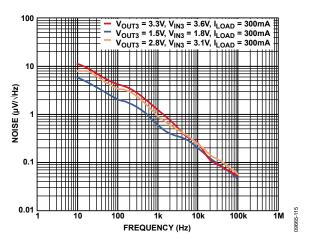
Figure 93. LDO2 Noise Spectrum Across Output Voltage,  $V_{IN} = V_{OUT} + 0.3 V$
