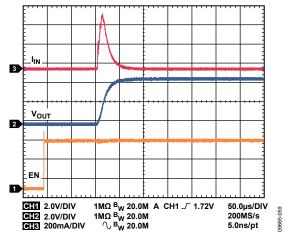
Figure 59. LDO1, LDO2 Startup,  $V_{OUT} = 4.7 V$ ,  $I_{OUT} = 5 mA$
