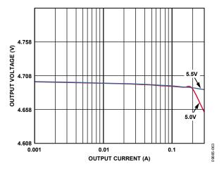
Figure 63. LDO1, LDO2 Load Regulation Across Input Voltage,  $V_{OUT} = 4.7 \text{ V}$
