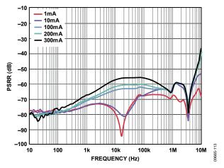
Figure 99. LDO1 PSRR Across Output Load,  $V_{\text{IN2}} = 5.0 \text{ V}, V_{\text{OUT2}} = 1.5 \text{ V}$
