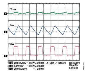
Figure 39. Typical Waveforms, V<sub>OUT1</sub> = 1.8 V, I<sub>OUT1</sub> = 30 mA, PWM Mode
