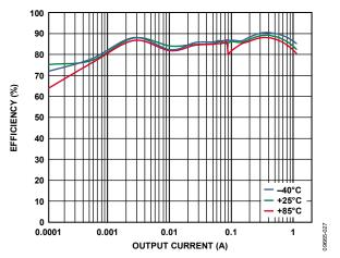
Figure 27. Buck Efficiency vs. Load Current, Across Temperature,  $V_{IN} = 5.0 \text{ V}, V_{OUTI} = 1.8 \text{ V}, \text{Auto Mode}$
