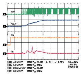
Figure 6. Buck Startup,  $V_{OUT1} = 3.3 \text{ V}$ ,  $I_{OUT2} = 20 \text{ mA}$
