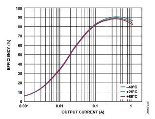
Figure 28. Buck Efficiency vs. Load Current, Across Temperature,  $V_{\text{IN}} = 5.0 \text{ V}, V_{\text{OUTI}} = 1.8 \text{ V}, PWM \text{ Mode}$
