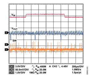
Figure 43. Buck Response to Line Transient, Input Voltage from 4.5 V to 5.0 V, V<sub>ΟUT1</sub> = 1.2 V, I<sub>ΟUT1</sub> = 5 mA, Auto Mode
