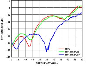
Figure 8. Return Loss vs. Frequency
