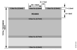
Figure 20. Probe Matrix Board Stack Up
