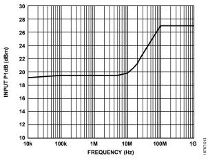
Figure 13. Input P1dB vs. Frequency (Low Frequency Detail)
