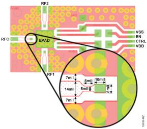
Figure 22. Impedance Matched Circuit
