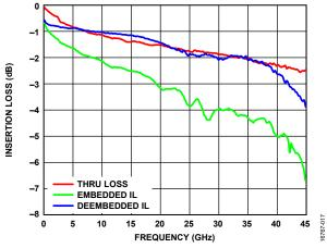
Figure 17. Insertion Loss vs. Frequency
