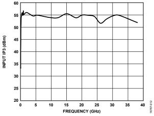
Figure 12. Input IP3 vs. Frequency
