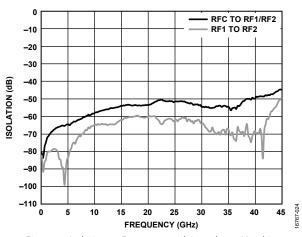
Figure 25. Isolation vs. Frequency, with Impedance Matching
