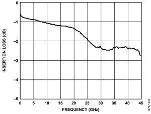
Figure 23. Insertion Loss vs. Frequency, with Impedance Matching
