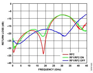
Figure 24. Return Loss vs. Frequency, with Impedance Matching
