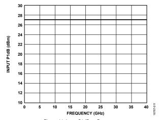
Figure 11. Input P1dB vs. Frequency
