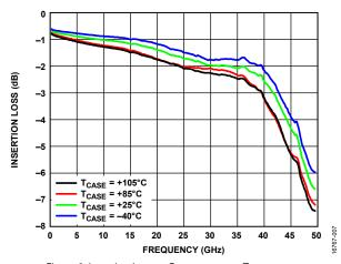
Figure 9. Insertion Loss vs. Frequency over Temperature
