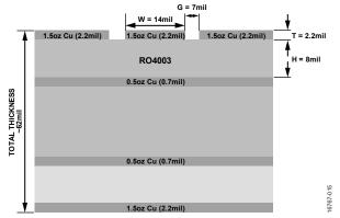
Figure 15. Evaluation Board Stack Up
