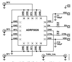
Figure 18. Simplified Evaluation Board Schematic
