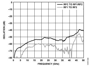
Figure 10. Isolation vs. Frequency
