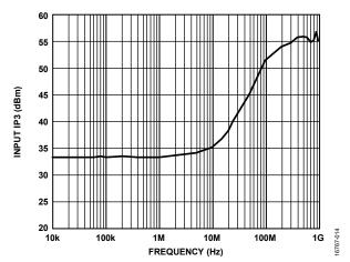
Figure 14. Input IP3 vs. Frequency (Low Frequency Detail)
