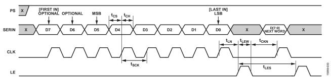
Figure 33. Serial Control Timing Diagram
