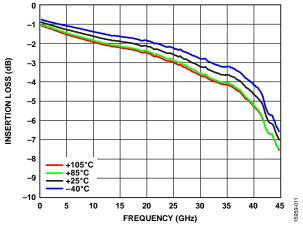
Figure 11. Insertion Loss vs. Frequency over Temperature Without Impedance
