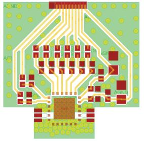
Figure 41. Probe Matrix Board Top View
