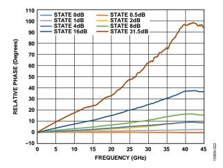
Figure 22. Relative Phase vs. Frequency (Major States Only) with Impedance
