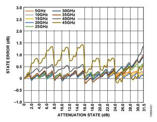
Figure 21. State Error vs. Attenuation State over Frequency with Impedance
