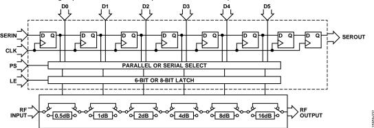
Figure 32. Simplified Circuit Diagram
