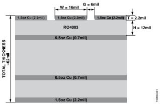
Figure 40. Probe Matrix Board Stackup, Cross Sectional View
