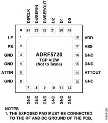
Figure 4. Pin Configuration
