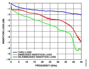
Figure 37. Insertion Loss vs. Frequency
