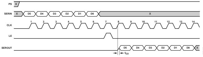
Figure 34. Serial Output Timing Diagram
