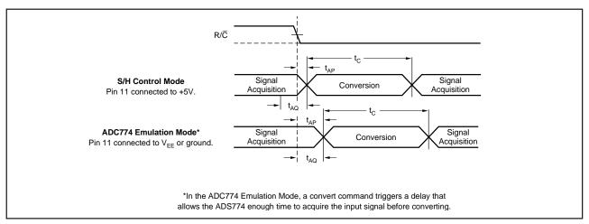
FIGURE 9. Signal Acquisition and Conversion Timing.
