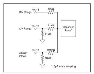
FIGURE 12. ADS774 Input Structure.
