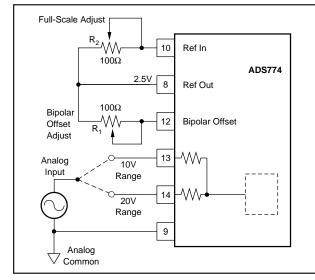
FIGURE 11. Bipolar Configuration.
