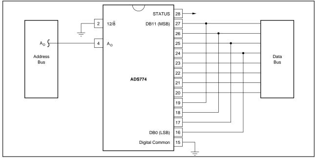
FIGURE 8. Connection to an 8-Bit Bus.
