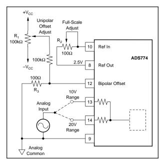
FIGURE 10. Unipolar Configuration.
