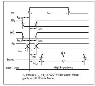
FIGURE 5. Conversion Cycle Timing.
