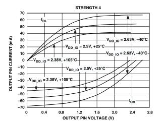
Figure 28. Typical Drive Currents at Strength 4
