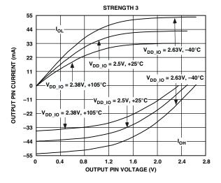
Figure 27. Typical Drive Currents at Strength 3
