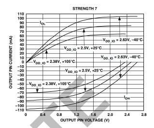
Figure 31. Typical Drive Currents at Strength 7
