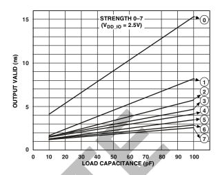
Figure 43. Typical Output Valid ( $V_{DD\ IO} = 2.5\ V$ ) vs. Load Capacitance at Max Case Temperature and Strength 0 to 7<sup>1</sup>
