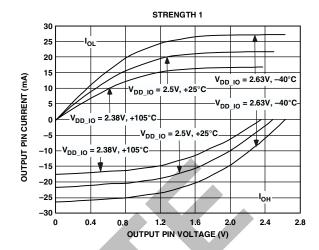
Figure 25. Typical Drive Currents at Strength 1
