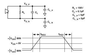
Figure 17. Link Ports—Differential Output Signals Transition Time
