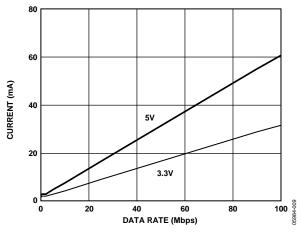
Figure 9. Typical ADuM3300 V<sub>DD1</sub> Supply Current vs. Data Rate for 5 V and 3.3 V Operation
