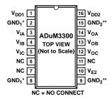
\*PIN 2 AND PIN 8 ARE INTERNALLY CONNECTED, AND CONNECTING BOTH TO GND<sub>1</sub> IS RECOMMENDED.
