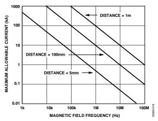
Figure 17. Maximum Allowable Current for Various Current-to-ADuM3300/ADuM3301 Spacings
