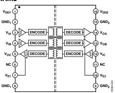
Figure 2. ADuM3301 Functional Block Diagram
