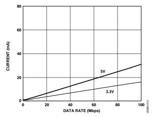
Figure 12. Typical ADuM3301  $V_{\rm DD2}$  Supply Current vs. Data Rate for 5 V and 3.3 V Operation
