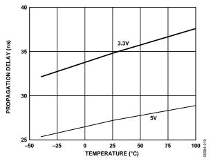
Figure 13. Propagation Delay vs. Temperature, C Grade
