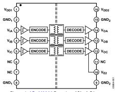
Figure 1. ADuM3300 Functional Block Diagram <sup>1</sup> Protected by U.S. Patents 5,952,849; 6,873,065; 6,903,578; and 7,075,329.
