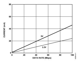
Figure 11. Typical ADuM3301 V<sub>DD1</sub> Supply Current vs. Data Rate for 5 V and 3.3 V Operation
