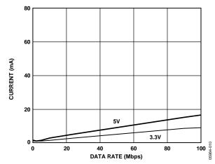
Figure 10. Typical ADuM3300 V<sub>DD2</sub> Supply Current vs. Data Rate for 5 V and 3.3 V Operation
