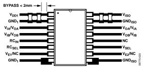
Figure 23. Recommended PCB Layout
