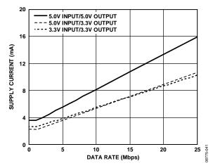
Figure 19. Typical I<sub>CHn</sub> Supply Current per Forward Data Channel (15 pF Output Load)
