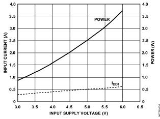
Figure 12. Typical Short-Circuit Input Current and Power vs. V<sub>DD1</sub> Supply Voltage
