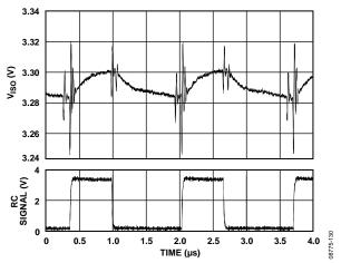
Figure 16. Typical Output Voltage Ripple at 90% Load, V<sub>ISO</sub> = 3.3 V
