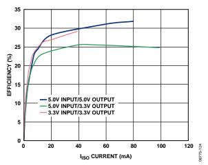
Figure 9. Typical Power Supply Efficiency in All Supported Power Configurations
