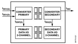
Figure 27. Power Consumption Within the ADuM620x
