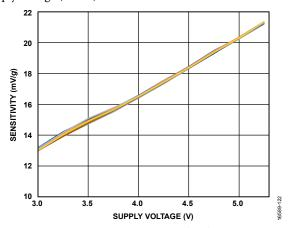
Figure 22. Sensitivity vs. Supply Voltage
