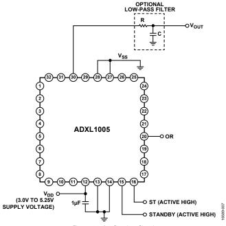
Figure 20. Application Circuit
