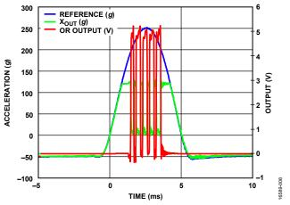
Figure 18. Response to Overload Condition, X<sub>OUT</sub> Delta is Difference from Midscale Voltage
