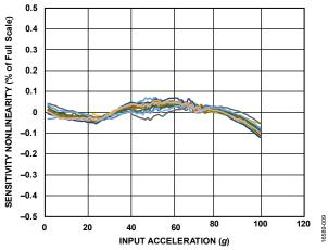
Figure 9. Sensitivity Nonlinearity vs. Input Acceleration
