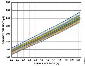
Figure 14. Standby Current vs. Supply Voltage
