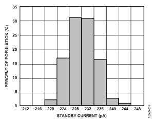
Figure 15. Standby Current Histogram at 25°C
