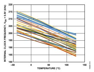
Figure 17. Internal Clock Frequency vs. Temperature at 5.0 V Supply Voltage ( $V_{\rm DD}$ )
