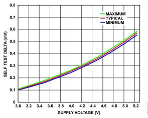
Figure 21. Typical Self Test Delta vs. Supply Voltage
