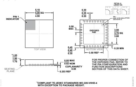
Figure 26. 32-Lead Lead Frame Chip Scale Package [LFCSP] 5 mm × 5 mm Body and 1.8 mm Package Height (CP-32-26) Dimensions shown in millimeters
