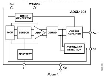
The integrated signal conditioning electronics enable such features as full electrostatic self test (ST) and an overrange (OR) indicator, useful for embedded applications. With low power and single-supply operation of 3.0 V to 5.25 V, the ADXL1005 also enables wireless sensing product design. The ADXL1005 is available in a 5 mm × 5 mm × 1.8 mm LFCSP package, and operates over the -40°C to +125°C temperature range.
