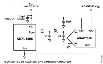
Figure 23. Application Circuit for the ADXL1005
