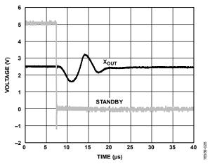
Figure 16. X<sub>OUT</sub> Output Recovery from Standby Mode to Measure Mode
