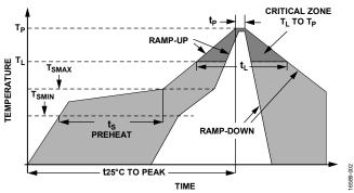
Figure 2. Recommended Soldering Profile
