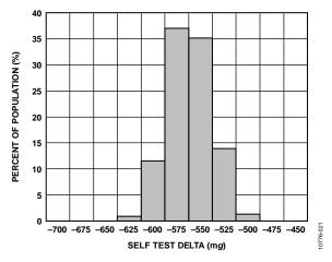
Figure 21. Y-Axis Self Test Response at  $25^{\circ}$ C,  $V_{S} = 2V$
