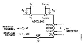
Figure 45. Using the INT2 Pin to Trigger Synchronized Sampling
