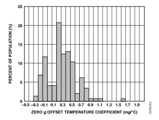
Figure 13. Z-Axis Zero g Offset Temperature Coefficient,  $V_S = 2 V$
