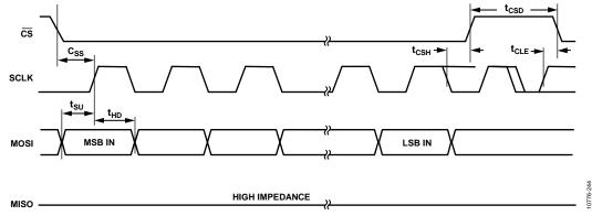
Figure 41. Timing Diagram for SPI Receive Instructions
