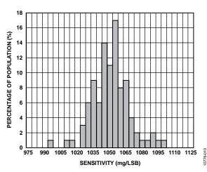
Figure 10. Z-Axis Sensitivity at 25°C,  $V_S = 2 V$ ,  $\pm 2 g$  Range
