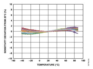
Figure 18. Y-Axis Sensitivity Deviation from  $25^{\circ}$ C vs. Temperature—16 Parts Soldered to PCB, ODR = 100 Hz,  $V_S$  = 2 V
