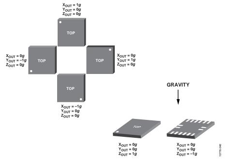
Figure 51. Output Response vs. Orientation to Gravity
