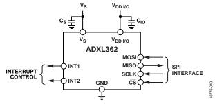
Figure 46. Recommended Bypass Capacitors
