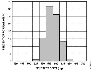
Figure 20. X-Axis Self Test Response at  $25^{\circ}$ C,  $V_{S} = 2 V$
