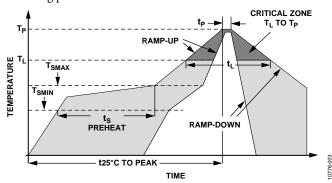
Figure 3. Recommended Soldering Profile
