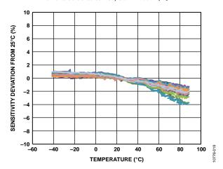
Figure 19. Z-Axis Sensitivity Deviation from  $25^{\circ}$ C vs. Temperature— 16 Parts Soldered to PCB, ODR = 100 Hz,  $V_S$  = 2 V
