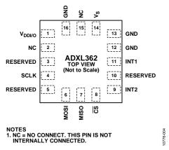
Figure 4. Pin Configuration (Top View)
