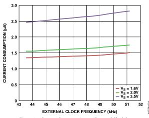
Figure 34. Current Consumption vs. External Clock Rate
