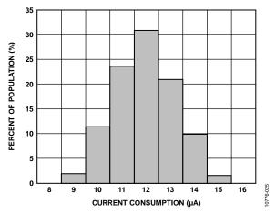
Figure 25. Current Consumption at 25°C, Ultralow Noise Mode,  $ODR = 100 \text{ Hz}, V_S = 2 \text{ V}$
