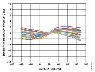
Figure 17. X-Axis Sensitivity Deviation from  $25^{\circ}$ C vs. Temperature— 16 Parts Soldered to PCB, ODR = 100 Hz,  $V_S = 2$  V
