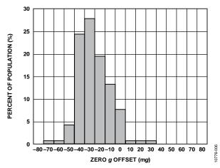
Figure 6. Y-Axis Zero g Offset at  $25^{\circ}$ C,  $V_S = 2 V$
