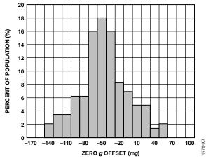
Figure 7. Z-Axis Zero g Offset at  $25^{\circ}$ C,  $V_S = 2 V$
