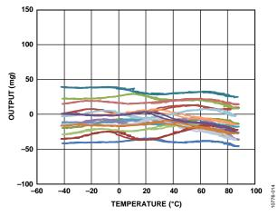
Figure 14. X-Axis Zero g Offset vs. Temperature— 16 Parts Soldered to PCB, ODR = 100 Hz,  $V_S = 2 V$
