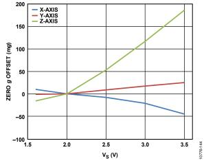
Figure 49. 0 g Offset vs. Supply Voltage
