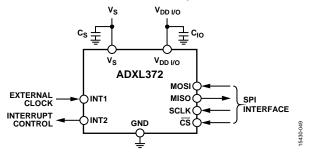
Figure 49. INT1 Pin as Input for External Clock
