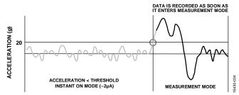
Figure 34. Instant On Mode Using Default Threshold
