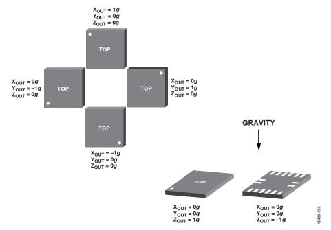
Figure 53. Output Response vs. Orientation to Gravity
