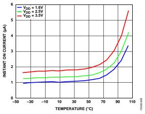
Figure 28. Instant On Current vs. Temperature
