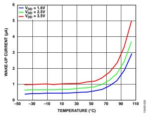
Figure 29. Wake-Up Current vs. Temperature
