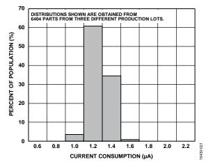
Figure 21. Current Consumption at 25°C, Instant On Mode,  $V_S = 2.5 \text{ V}$
