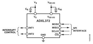
Figure 48. Recommended Bypass Capacitors
