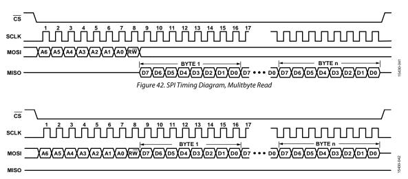
Figure 43. SPI Timing Diagram, Multibyte Write
