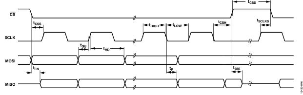
Figure 39. SPI Timing Diagram
