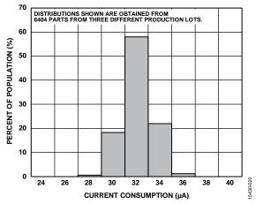
Figure 20. Current Consumption at 25°C, Low Noise Mode, 3200 Hz Output Data Rate,  $V_S = 2.5 \text{ V}$
