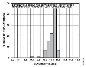
Figure 8. Y-Axis Sensitivity at 25°C,  $V_S = 2.5 \text{ V}$
