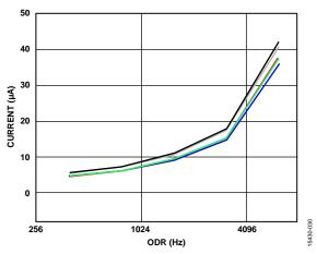
Figure 30. Measurement Mode Current vs. ODR for Five Parts
