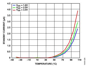
Figure 26. Standby Current vs. Temperature
