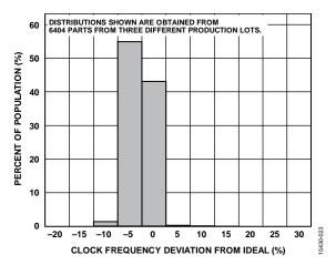
Figure 23. Clock Frequency Deviation from Ideal at 25°C, ODR = 3200 Hz,  $V_S$  = 2.5  $V_S$
