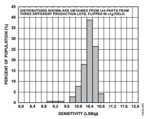
Figure 9. Z-Axis Sensitivity at 25°C,  $V_S = 2.5 \text{ V}$
