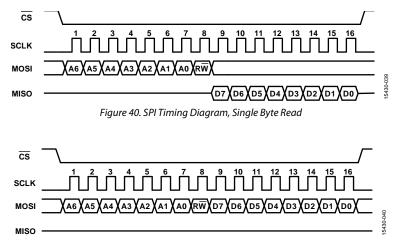
Figure 41. SPI Timing Diagram, Single Byte Write
