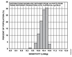
Figure 7. X-Axis Sensitivity at 25°C,  $V_S = 2.5 \text{ V}$
