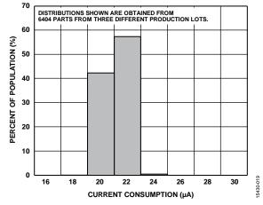
Figure 19. Current Consumption at 25°C, Normal Mode, 3200 Hz Output Data Rate,  $V_S = 2.5 \text{ V}$
