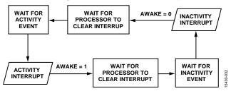
Figure 32. Flowchart Illustrating Activity and Inactivity Operation in Linked Mode
