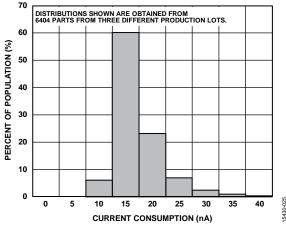
Figure 25. Current Consumption at 25°C, Standby Mode,  $V_S = 2.5 \text{ V}$
