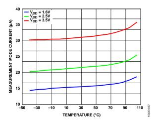
Figure 27. Measurement Mode Current vs. Temperature
