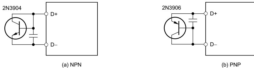
Figure 88. Remote Temperature Sensor Using Transistor
