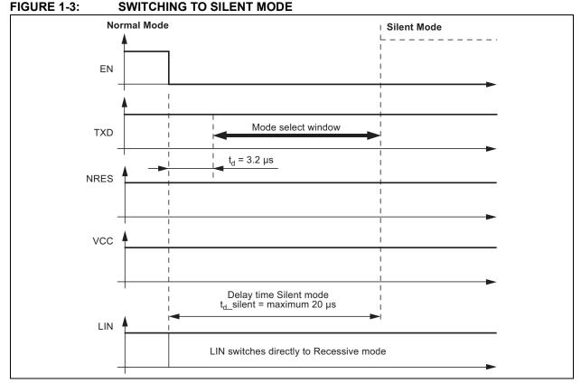
In Silent mode, the internal slave termination between the LIN pin and VS pin is disabled to minimize the current consumption in case the pin LIN is shortcircuited to GND. Only a weak pull-up current (typically 10  $\mu$ A) between the LIN pin and VS pin is present. Silent mode can be activated independently from the current level on pin LIN.
