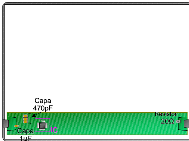
Figure 41. Layout example for ESD protection
