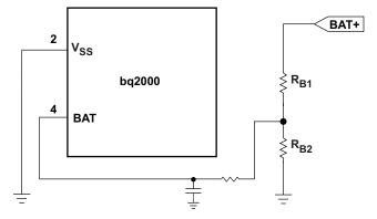
Figure 3. Battery Voltage Divider and Filter
