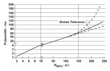
Figure 8. Relationship Between Trickle Pulse-Width and Value of R<sub>MTO</sub>
