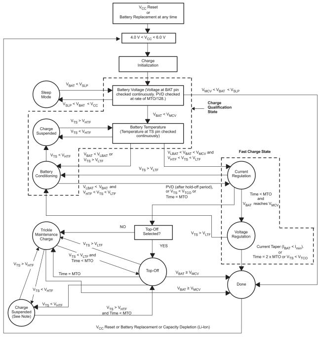
NOTE: If  $V_{TS} < V_{TCO}$  at any time, may only return to Trickle Maintenance Charge state and not to Top-Off.
