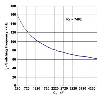
Figure 10. Switching Frequency vs Capacitance
