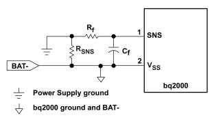
Figure 9. Current-Sensing Circuit
