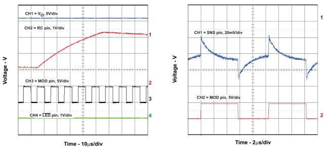
Figure 16. bq2000 in Fast Charge
