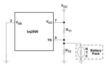
Figure 6. Temperature Monitoring Configuration
