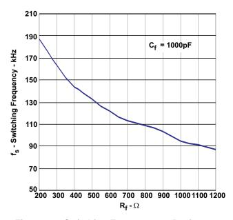
Figure 11. Switching Frequency vs Resistance
