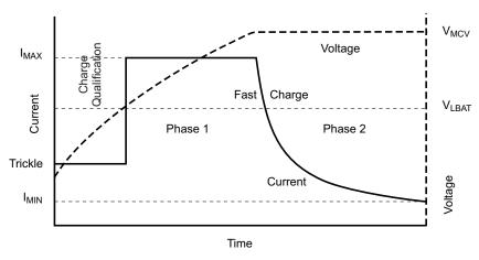
Figure 4. Lithium-Ion Charge Algorithm
