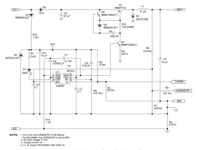
Figure 7. Single-Cell Li-Ion, 3-Cell NiCd/NiMH 1A Charger
