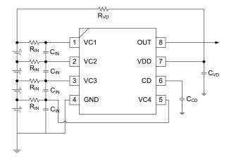
Figure 7. 4-Series Cell Configuration
