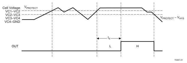
Figure 4. Timing for Overvoltage Sensing
