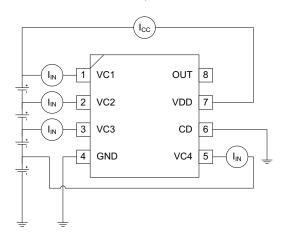
Figure 3. I<sub>CC</sub>, I<sub>IN</sub> Measurement
