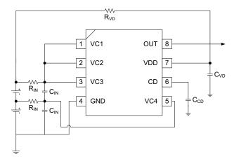
Figure 5. 2-Series Cell Configuration
