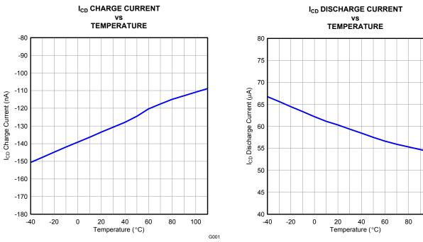
Figure 1. I<sub>CD</sub> Charge Current
