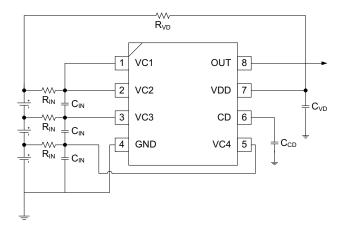
Figure 6. 3-Series Cell Configuration
