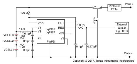
Figure 9-2. 3-Series BQ2961 and BQ2962 Schematic
