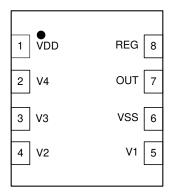
Figure 6-2. 2-Series to 4-Series BQ2962 (Top View)
