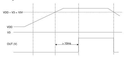
Figure 8-3. Timing for Customer Test Mode
