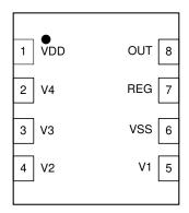
Figure 6-1. 2-Series to 4-Series BQ2961 (Top View)
