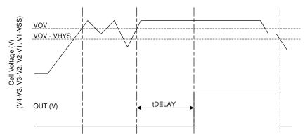
Figure 8-1. Timing for Overvoltage Sensing for OUT
