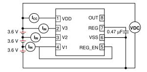
Figure 8-4. Configuration for Integrated Circuit Current Consumption Test
