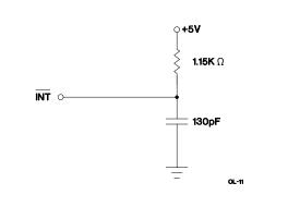
Figure 6. Output Load B
