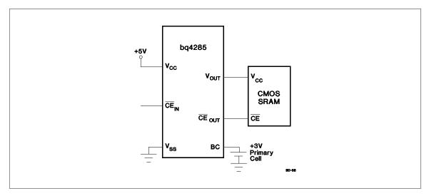
Figure 4. External RAM Hookup to the bq4285 RTC
