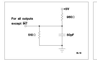
Figure 5. Output Load A
