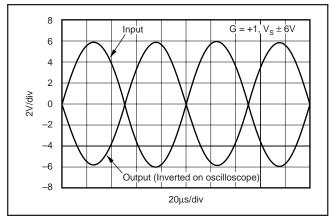
FIGURE 2. Rail-to-Rail Input and Output.
