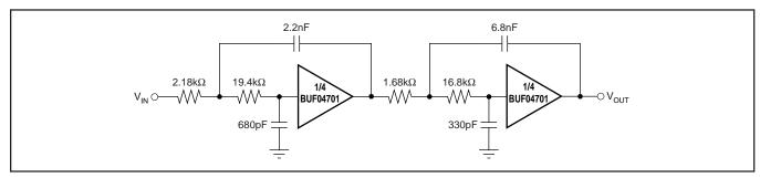
FIGURE 7. BUF04701 Configured as a 4-Pole Sallen-Key Butterworth Low-Pass Filter.
