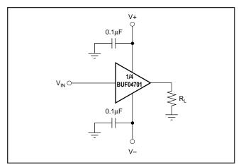
FIGURE 1. Basic Connections.
