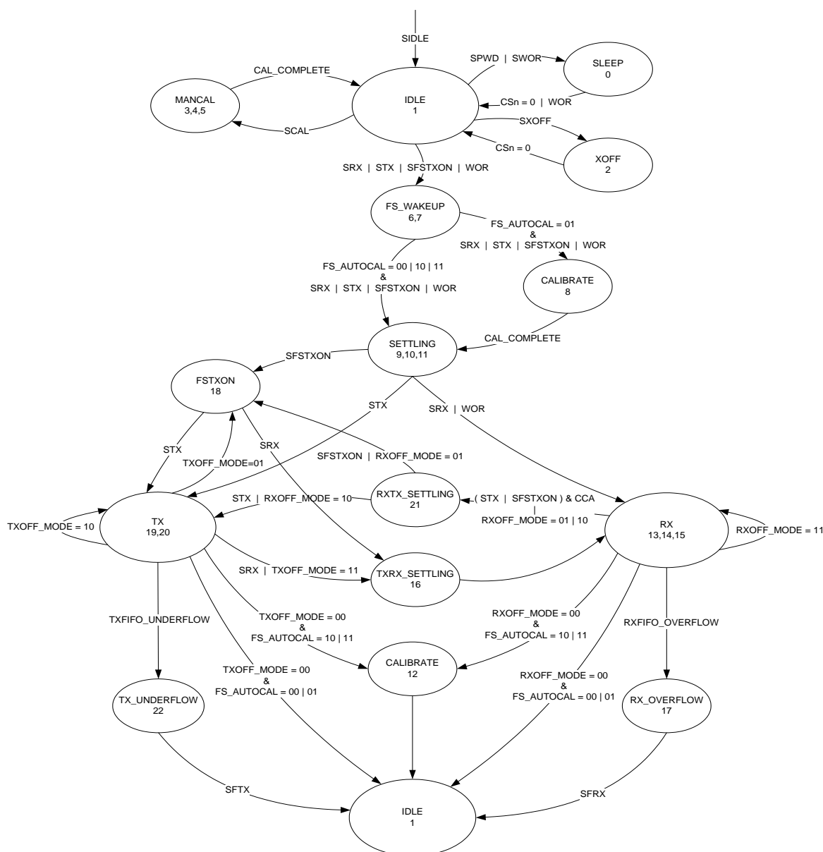
Figure 25: Complete Radio Control State Diagram
