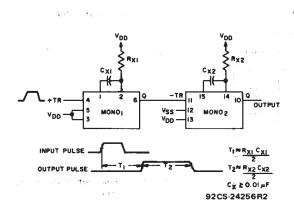
Fig. 15 - Pulse delay.
