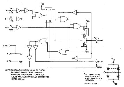
Fig. 4 — CD4098B logic diagram.
