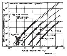
Fig. 9 – Typical external capacitance vs. pulse width.
