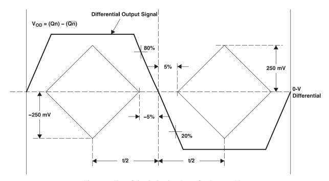
Figure 2. Test Criteria for  $f_{clk}$ , Duty Cycle,  $t_r$ ,  $t_f$ ,  $V_{OD}$
