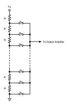
Figure 29. DAC Resistor String
