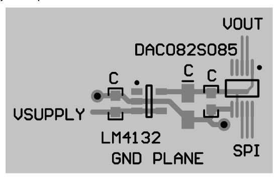
Figure 41. DAC082S085 Layout Example
