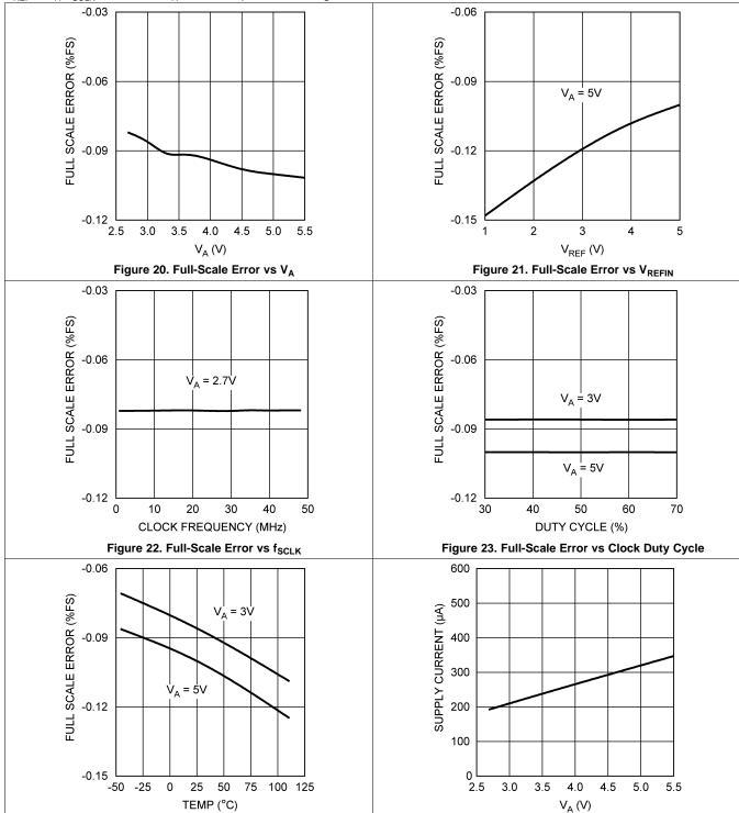
Figure 24. Full-Scale Error vs Temperature
