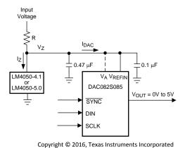
Figure 38. The LM4050 as a Power Supply
