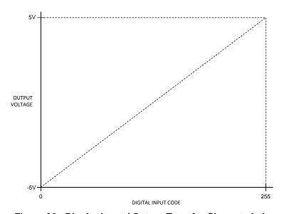
Figure 36. Bipolar Input / Output Transfer Characteristic
