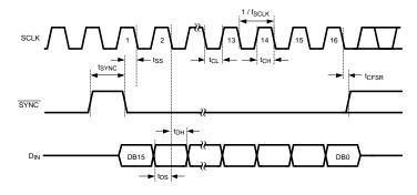
Figure 1. Serial Timing Diagram
