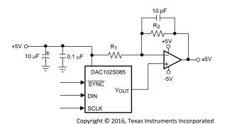
Figure 35. Bipolar Operation
