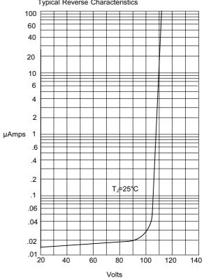
Instantaneous Reverse Leakage Current - MicroAmperesersus Percent Of Rated Peak Reverse Voltage - Volts
