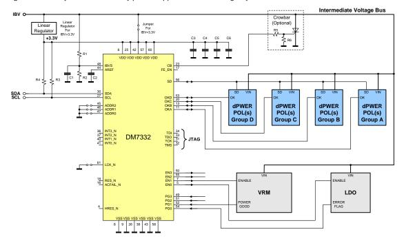
Figure 49. Multi-dPOL Power System Diagram
