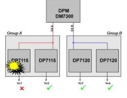
Figure 31. No Group Fault Propagation
