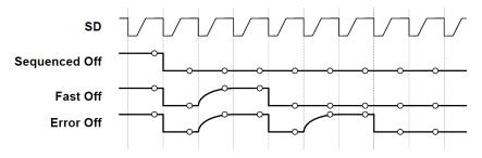
Figure 35. OK Severity Encoding Waveforms
