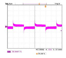
Figure 44. Transient Response with Regulation set to 3.72mV/A
