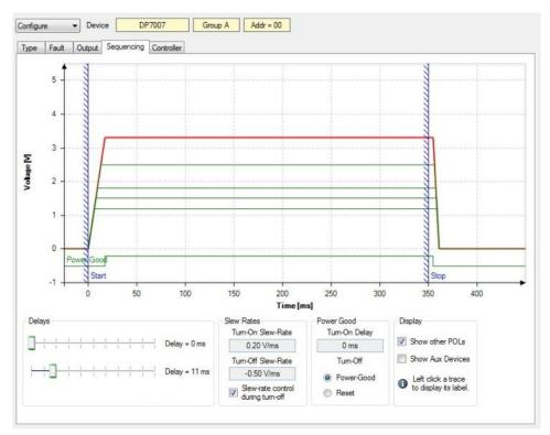
Figure 11. dPOL Configure Sequencing Window
