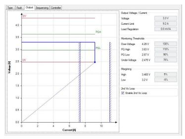
Figure 6. Output Configuration Window
