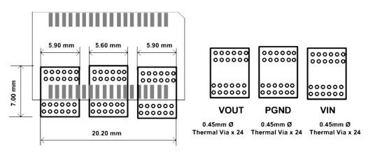
Recommended via diameter is 0.45mm Barrel wall plating of > 25um Pitch <1.00mm
