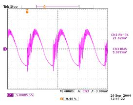
Figure 40. Output Voltage Noise, Full Load, No Interleave
