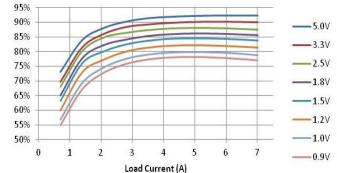
Figure 3. Efficiency vs. Load. Vin=12V, Fsw=500kHz
