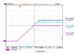
Figure 16. Tracking Turn-On. Rising Slew Rate is programmed at 0.5V/ms for each output.
