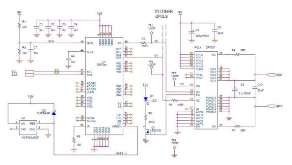
Figure 50. Typical Application with Digital Power Manager and I2C Interface
