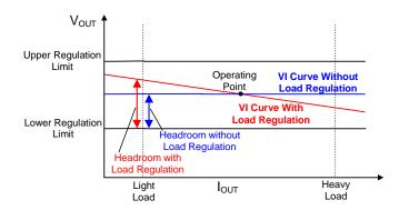
Figure 8. Optimal Voltage Positioning Concept
