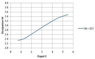
Figure 5 Dissipation vs Voltage. Iout=7A, Fsw=500kHz
