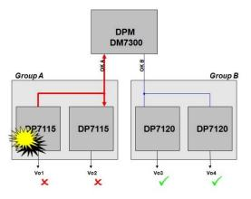
Figure 33. Intra Group Fault Propagation
