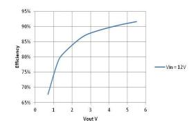
Figure 4. Efficiency vs. Output Voltage, Iout=7A, Fsw=500kHz
