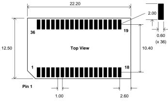
Figure 54. Recommended PCB Pad Sizes
