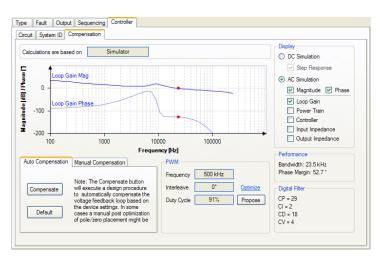
Figure 36. PWM Controller Window
