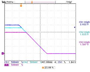
Figure 21. Tracking Turn-Off. Falling Slew Rate is Programmed at 0.5V/ms
