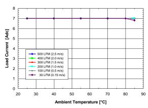
Figure 2. Available output current vs. ambient air temperature and airflow rates for converter DP7007G mounted horizontally with air flowing from input to output, MOSFET temperature ≤ 120 °C, Vin = 12 V, Vout = 5 V, and Fsw= 1MHzw
