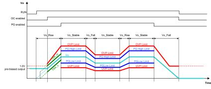
Figure 25. Protection Enable Conditions
