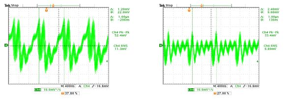
Figure 38. Input Voltage Noise, No Interleave
