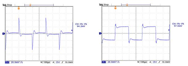
Figure 9 Transient Response with Regulation set to 0 mV/A
