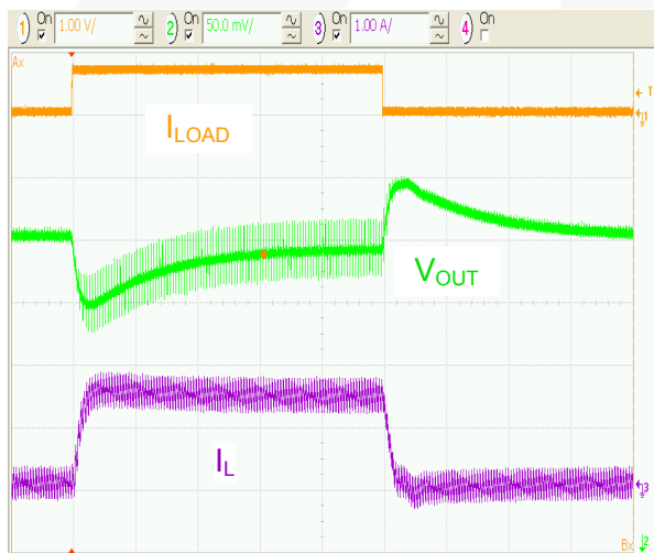
Figure 6. Load Transient Response, 1.2V OUT (100mA to 150mA, 20μs/div)
