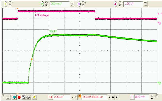
Figure 30. Startup / Shutdown, No Load, V_{OUT}=0.9\text{ V}
