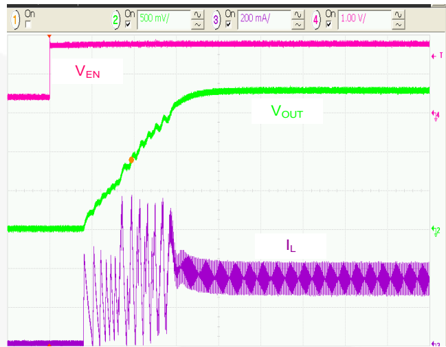
Figure 18. Soft-Start, R_{LOAD} = 6\Omega , 20 \mu s/div.
