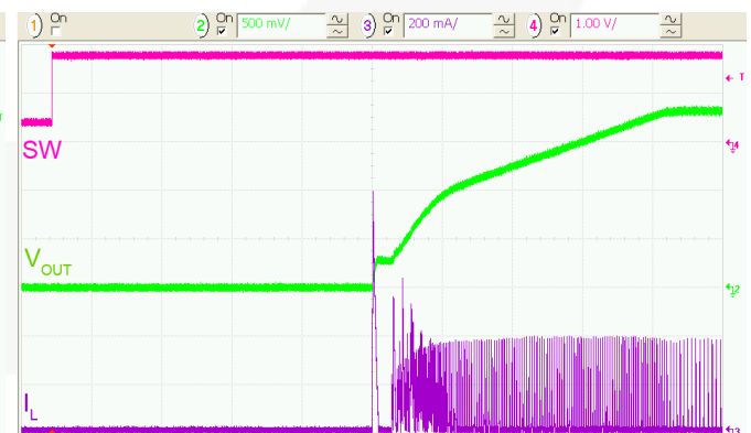
Figure 38. Soft-Start, R_{LOAD} = 50\ \Omega , 20\ \mu\text{s}/\text{div} .
