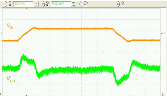
Figure 21. Line Transient 3.3 V_{IN} to 3.9 V_{IN} , 250 mA Load, 10 \mu\text{s}/\text{div} .
