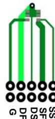
b. 175\text{ }^\circ\text{C/W} when mounted on a minimum pad of 2 oz copper
